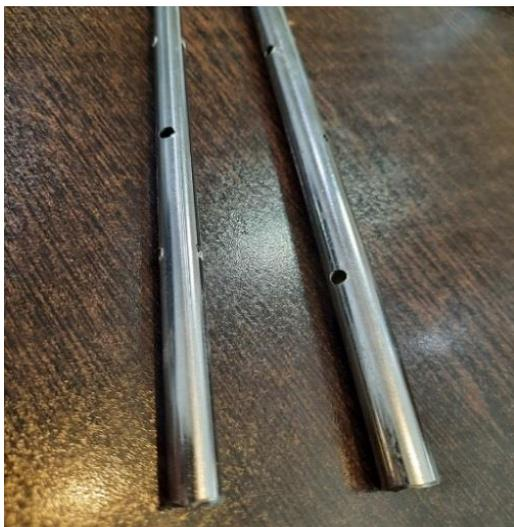
Figure 7. Non-grouted micropiles used in the tests
