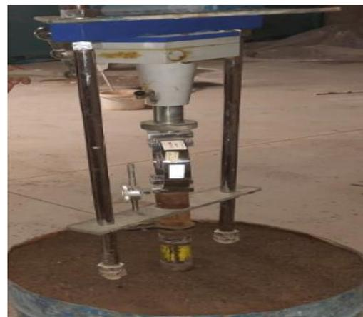
Figure 6. Plate loading tests set
