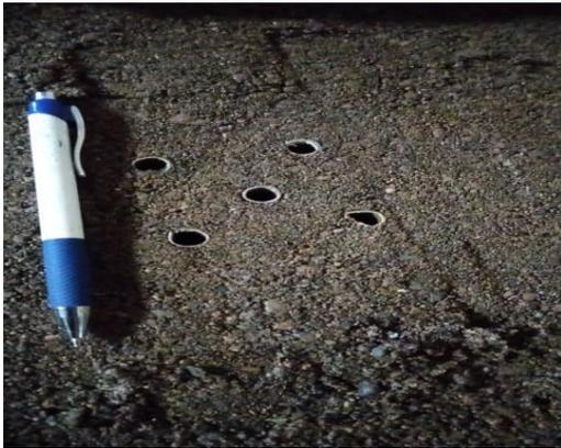
Figure 14. Five bio-micropile arrangement
