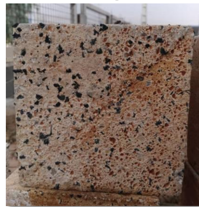
(b) Specimen with 15% CTR
