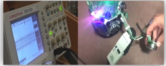
Figure 11. Set-up of the prototype BLDC motor
