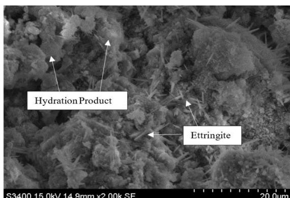
Figure 5. SEM image for C10QD mix after 7 days of curing
