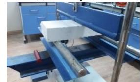
(e) Modulus of rupture test
