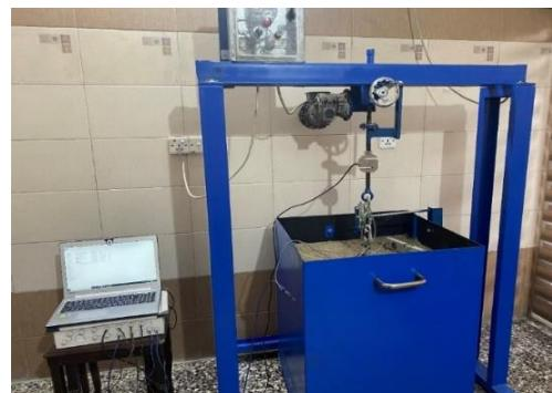
**Figure 2.** Under-reamed pile test
