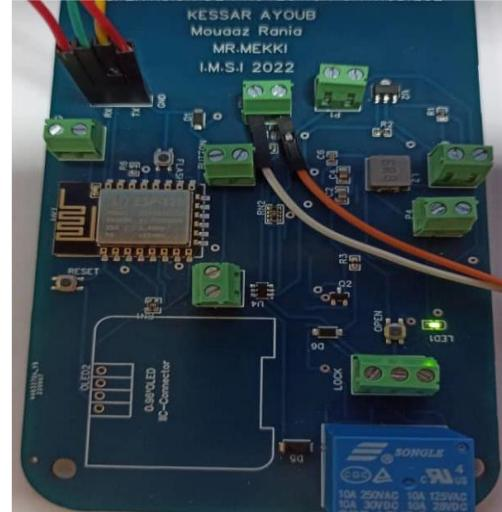
Figure 13. The relay works correctly by lighting the Led
