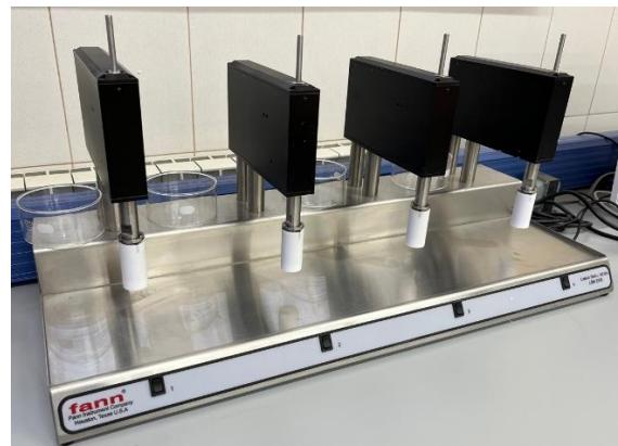
**Figure 3.** Linear clay swelling tester LSM 2100 (compiled by the authors)
