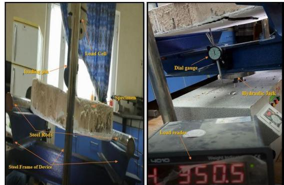
**Figure 6.** Test setup image
