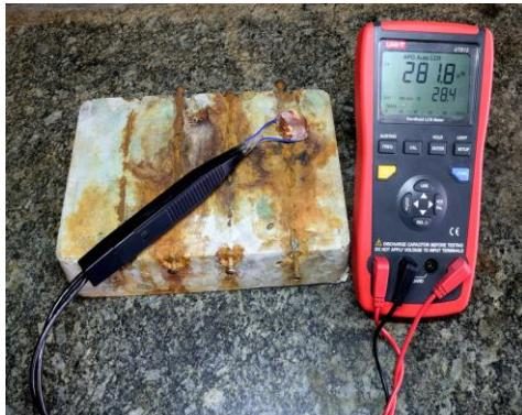
**Figure 7.** Schematics of corrosion monitoring of rebars in reinforced concrete by a LCR meter
