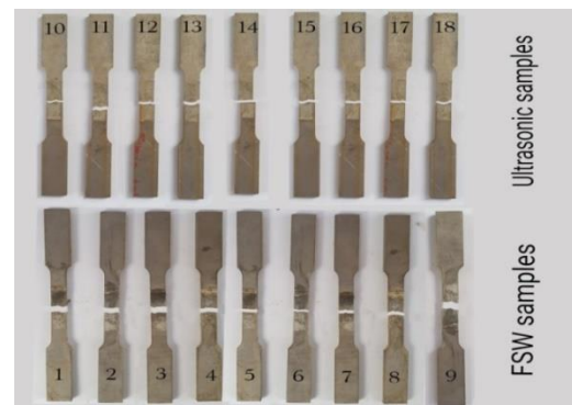
Figure 6. Welded samples after tensile test
