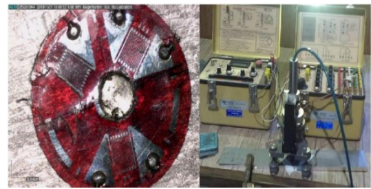
Figure 24. Central drilling test with strain gauge installation
