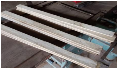
Plate 1. Wood laminates for glue lamination
