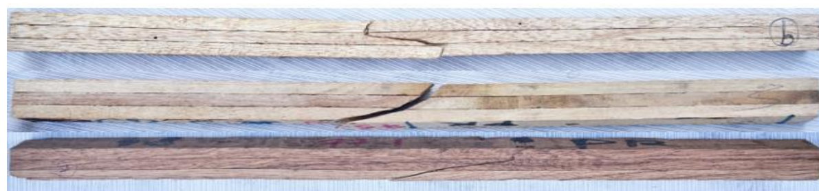
Plate 5. Cross grain tension failure in glulam beams
