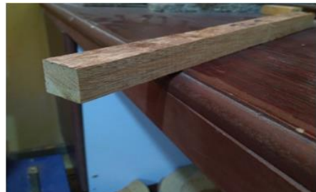
Plate 3. Finished glued laminated beam ready for testing
