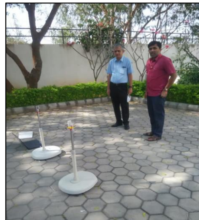
Figure 1. Outdoor experimental setup consisting of PVC stands, IoT modules and system
