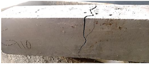
Figure 9. Specimen G10 for example after failure
