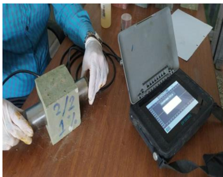
Figure 4. UPV test by using (S-wave) transducer
