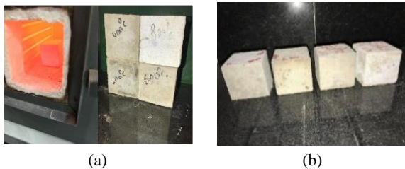
Figure 5. The appearance of RS-ECC after temperature exposure: A 28 days; B 90 days
