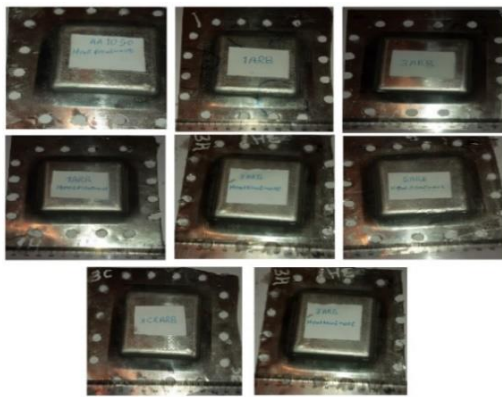
Figure 9. Samples produced by experimental SPIF processes
