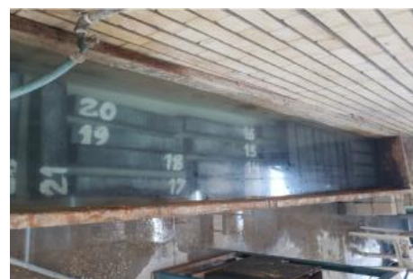
Figure 2. Curing stage of fiber concrete beams
