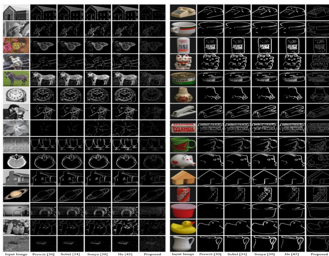
Figure 13. Edge detection results applied to images in Figure 12
