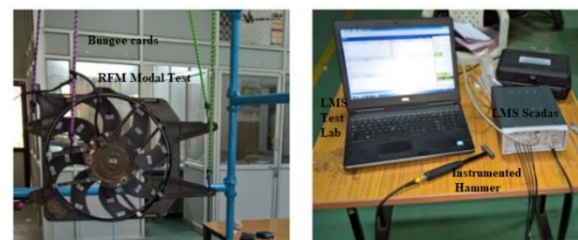
Figure 3. Experimental setup for spectral test
