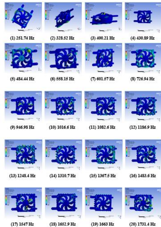
Figure 13. Modal parameters obtained from finite element analysis of shroud
