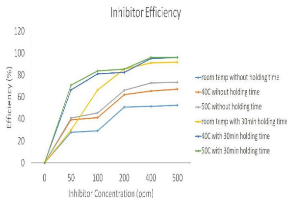
Figure 4. Inhibitor efficiency of API 5L in 0.1 M HCl and various Eucheuma inhibitor at different temperatures
