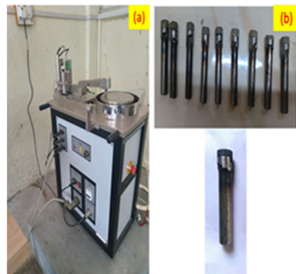
Figure 2. (a) Pin on Disc test set up (b) Pins
