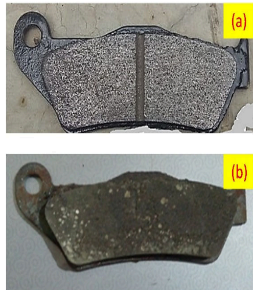
Figure 10. Brake pads (a) Commercial (b) Newly developed
