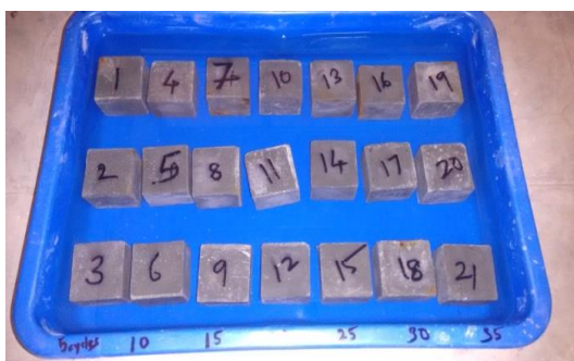
Figure 2. Specimens immersed in \text{Na}_2\text{SO}_4 solution
