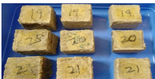
Figure 5. RPC Samples with 7 days exposure
