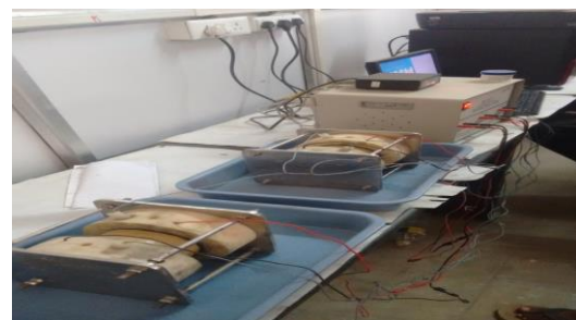
Figure 3. Rapid Chloride ion Penetration Test
