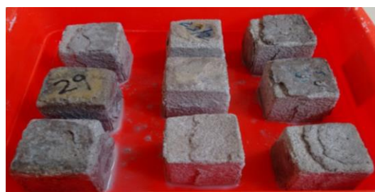
Figure 7. Scaling of RPC Samples with 60 days
