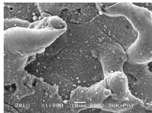
Figure 7. Micro- craks of machined surface
