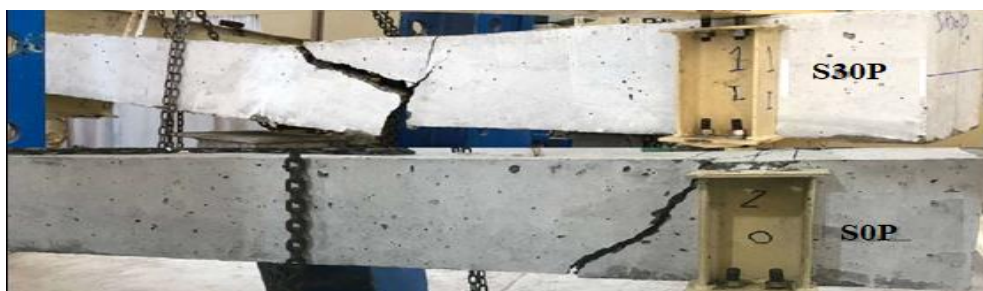
Figure 10. Failure shape of plain concrete beams
