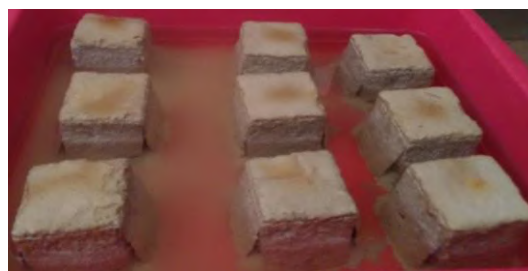
Figure 8. Spalling of RPC Samples with 60 days exposure
