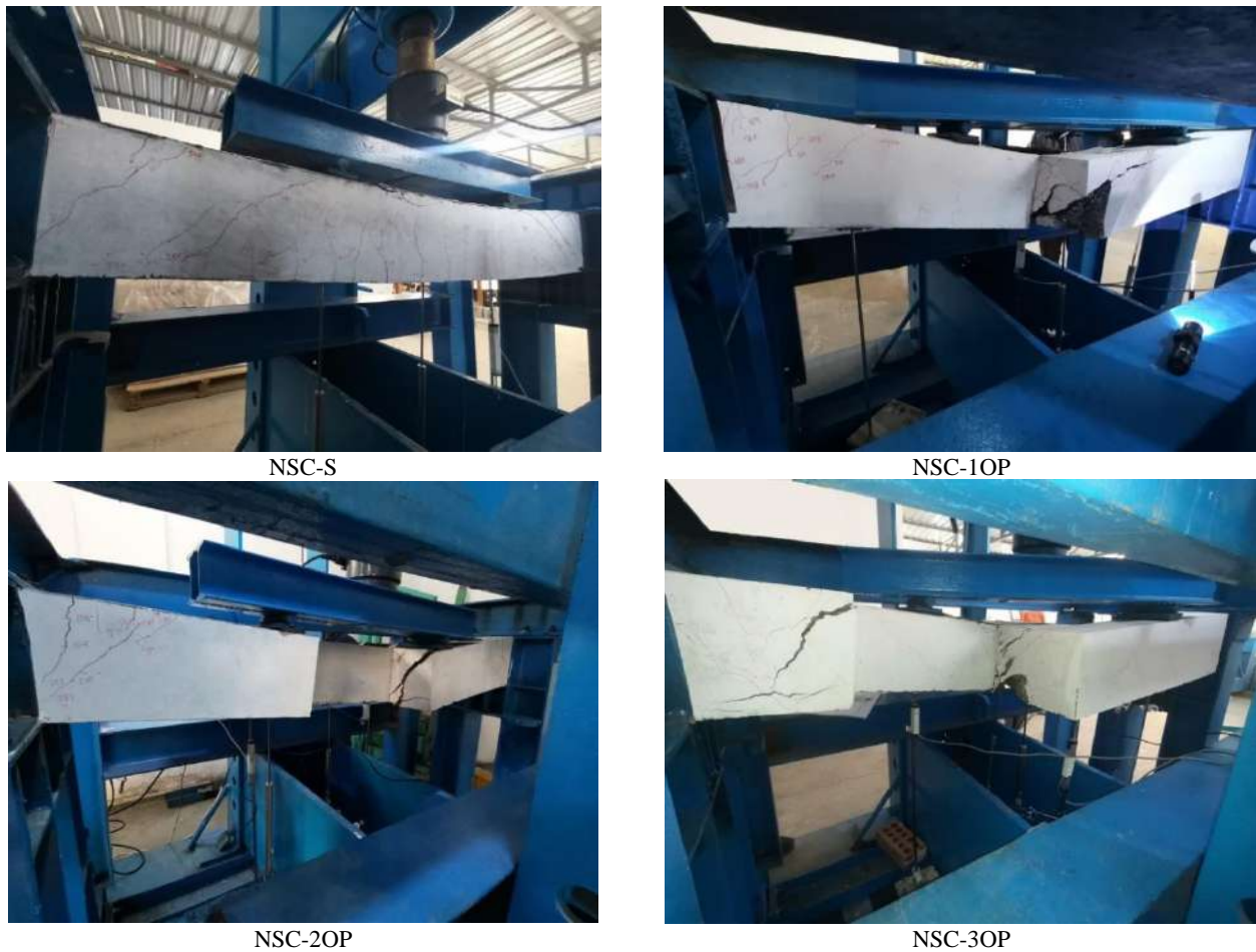
Figure 7. Specimens behavior at the failure load
