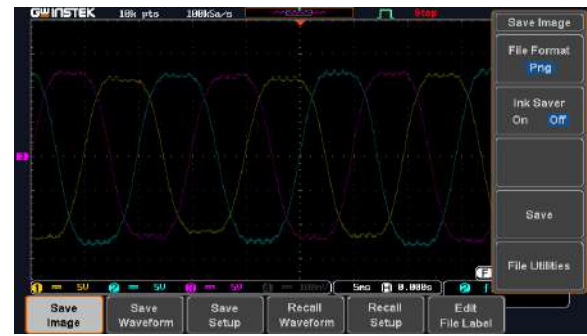
Figure 7. Back EMF waveform of (a) the analyzed result and (b) the experimental result
