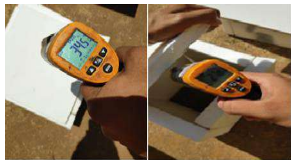
Figure 5. Temperature testing inside and outside of tile
