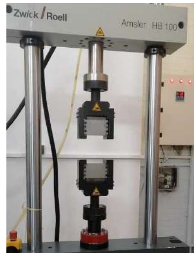
Figure 1. Zwick/roell amsler HB100 machine
