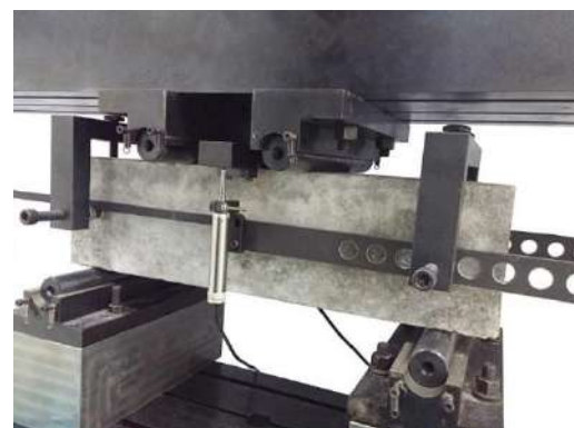
Figure 4. Fibrous concrete prism under flexural testing
