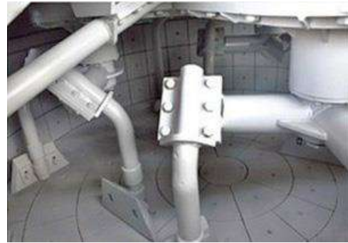
(a) Centrifuge mixer (inside view)
