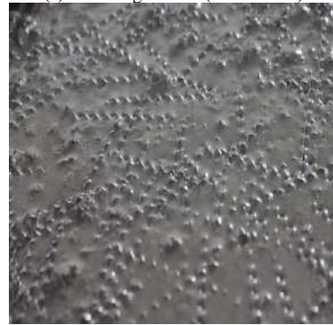
(b) Uniform distribution fibres after mixing procedure Figure 2. Mixer and a sample of a mixed matrix
