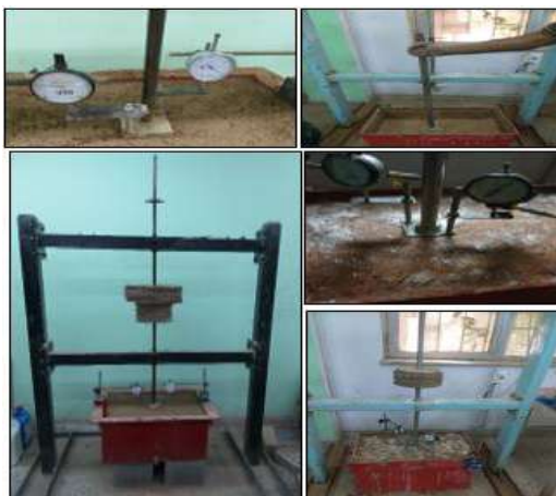
Figure 7. Performing loading on gypseous soil pressure
