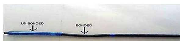
Figure 7. PSWC rebar with bonded and un-bonded regions
