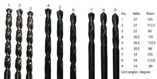
Figure 3. Standard drilling tool (Diameter: 3.5 mm) with different point and helix angles
