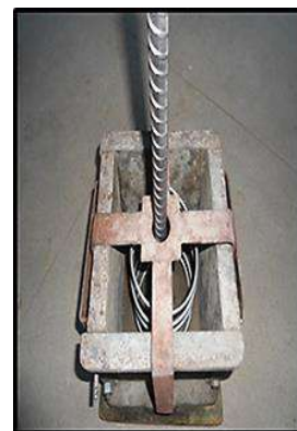
Figure 3. Arrangement of mould for casting pull-out specimen
