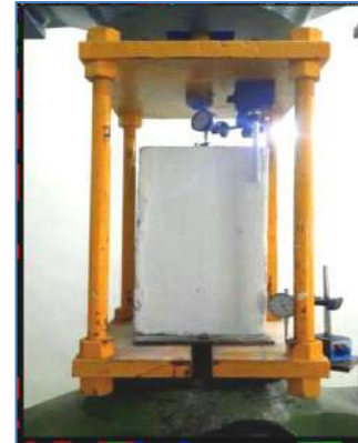
Figure 9. Pull-out test in progress
