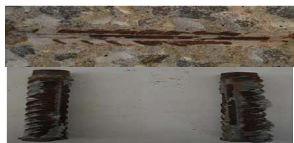
Figure 14. Condition of concrete and coated rebar at the end of the test
