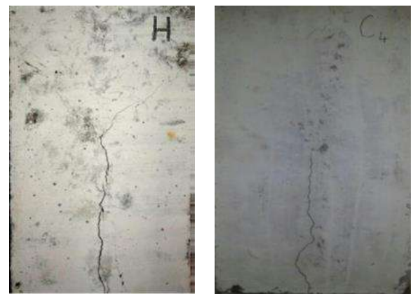
Figure 12. Crack pattern in beam-end specimens
