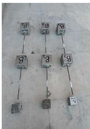
Figure 4. Casted BIS pull-out specimens
