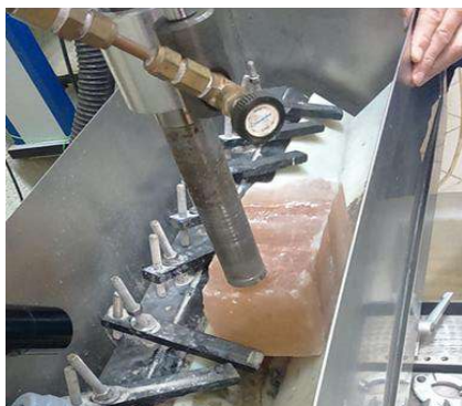
Figure 1. Preparation of NaCl samples using coring machine
