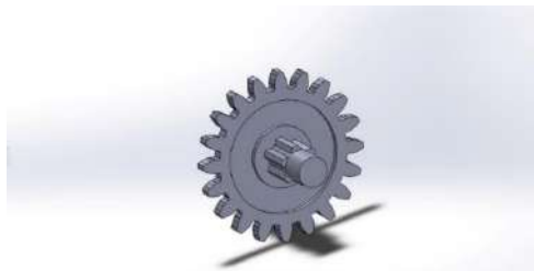
Figure 3. Spur gear model with the shaft in SOLIDWORKS 3D environment
