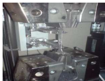
Figure 8. ZWICK tester in welding test mode
