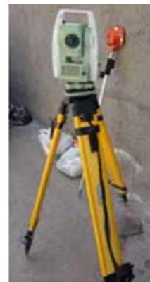
Figure 3. Topographic camera of Leica series of total station TS02 model
