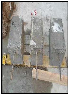
Figure 8. Casted beam-end specimens
