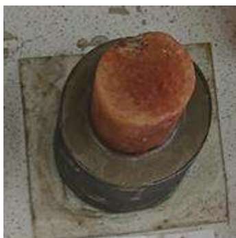
Figure 2. Cylindrical salt sample inside cement
