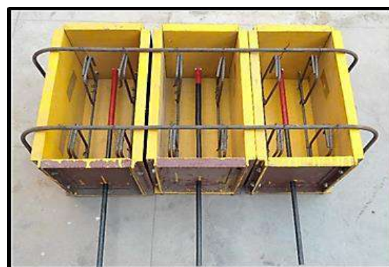
Figure 6. Arrangement of mould for casting beam-end specimens
