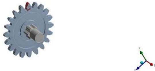
Figure 5. Application of 350 N force on a gear tooth
