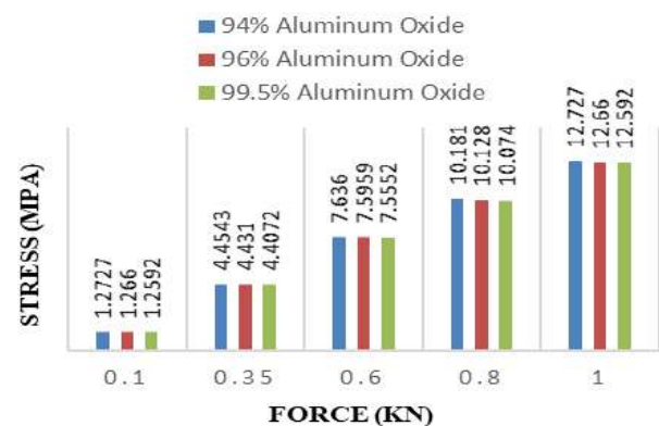
Figure 9. Stress results for 94% aluminum oxide, 96% aluminum oxide, and 99.5% aluminum oxide composite material gears
