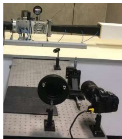
Figure 3. The Schlieren arrangement for the small test section wind tunnel
