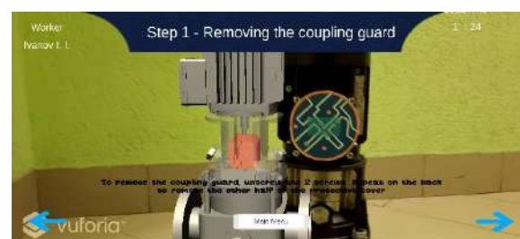
Figure 10. Removing two halves of the clutch
