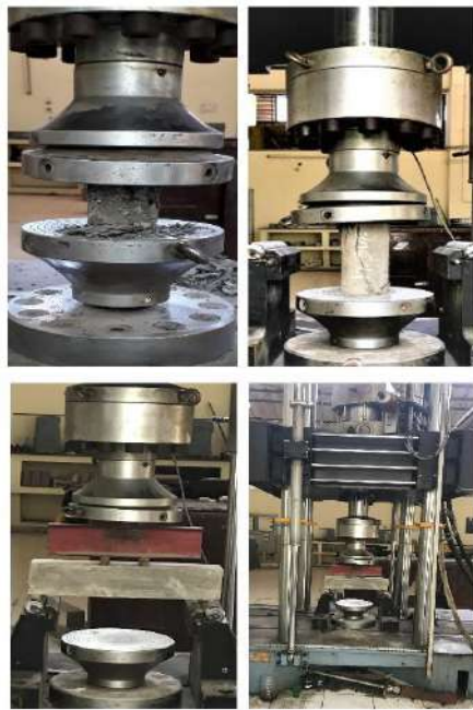
Figure 2. 1000kN servo-controlled test setup
