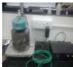
Figure 1. Shrinkage Cone Test setup
