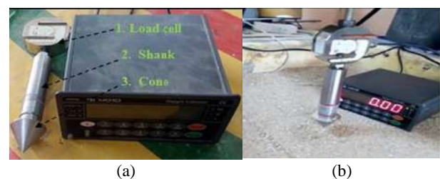
Figure 3. Measuring device for soil shear resistance; a. Components, b. Measuring device
