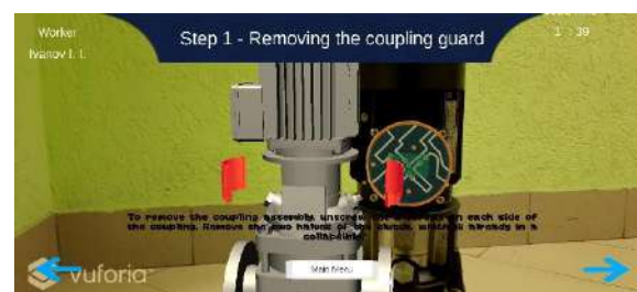
Figure 9. Removing the coupling guard
