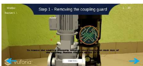
Figure 8. Unscrew two screws of coupling guard
