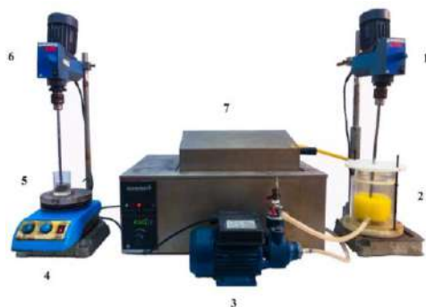
Figure 1. The main setup and its various components; (1, 6) Mixtures (2) Reactor T_1 (3) Pump (4) Heater (5) Reactor T_2 (7) Waterbath
