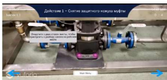
Figure 6. Removing pump from laboratory unit
