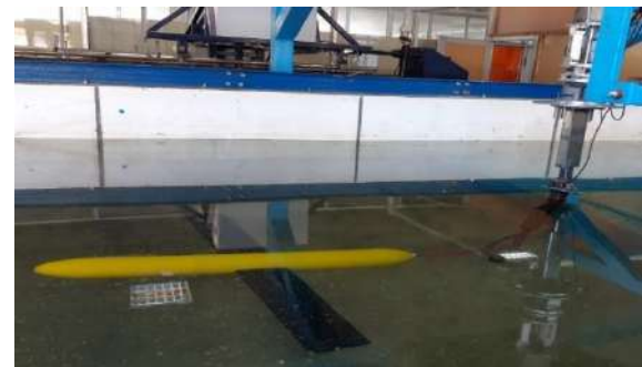
Figure 4. Underwater glider specimen made in a towing tank test
