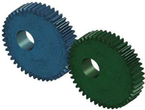
Figure 4. The meshing finite element model of elliptic cylinder gear
