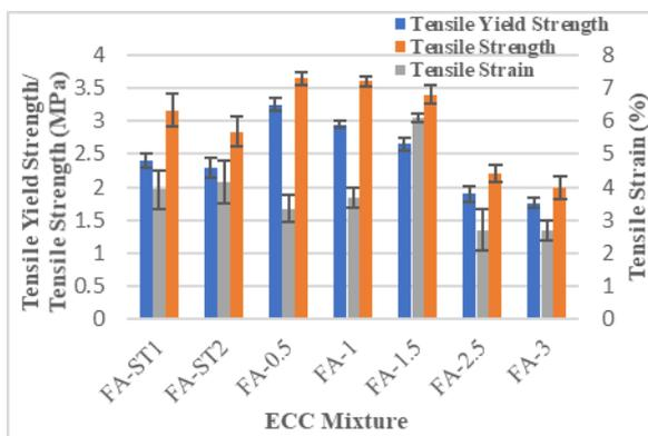
Figure 8. Comparison of ECC tensile behavior
