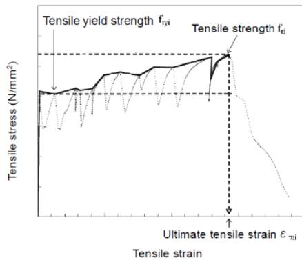
Figure 7. Definition of ECC characteristics
