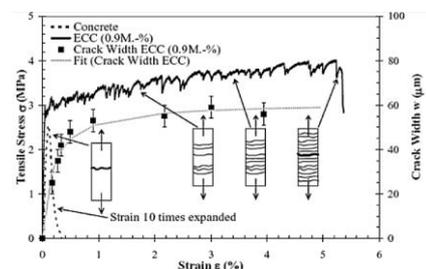
Figure 1. Comparison of the tensile behavior of concrete and ECC [2]
