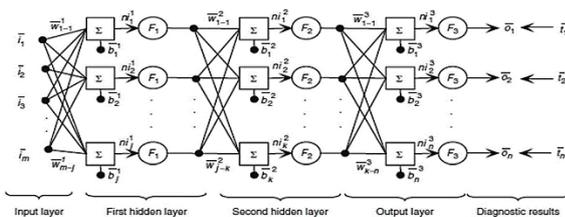
Figure 9. ANN model with one input, two hidden and one output layers [29, 30]
