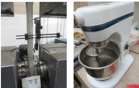
Figure 4. Producing and test set-up of ECC specimens [15]
