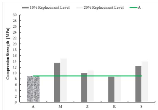
Figure 1. 7-day compressive strength of the specimen containing different types of pozzolans
