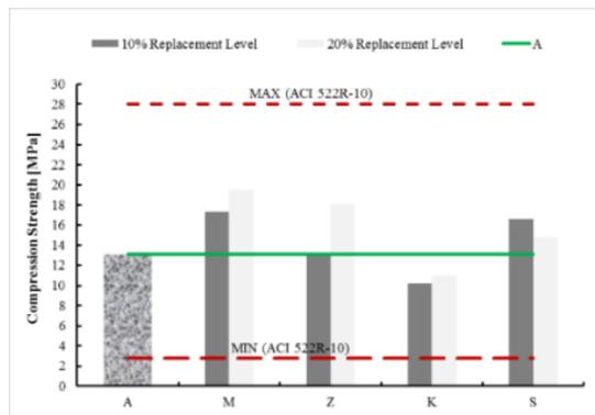
Figure 2. 28-day compressive strength of the specimen containing different types of pozzolans
