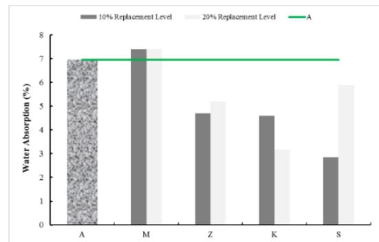
Figure 5. Water absorptions of the specimens containing different types of pozzolans at the age of 7 days
