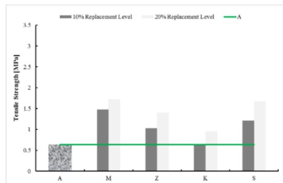
Figure 3. 7-day tensile strength of the specimen containing different types of pozzolans
