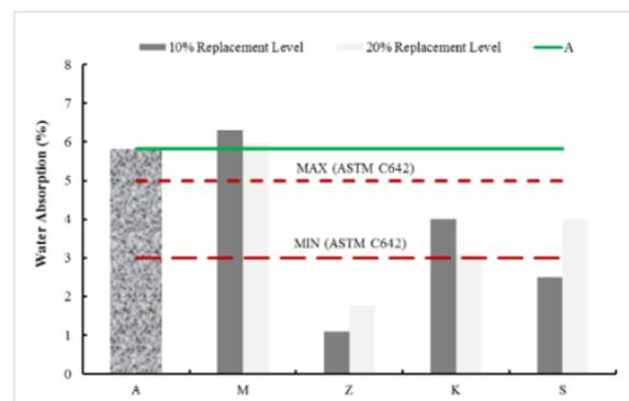
Figure 6. Water absorptions of the specimens containing different types of pozzolans at the age of 28 days
