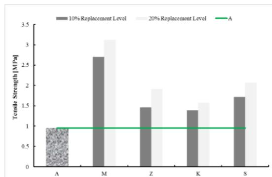
Figure 4. 28-day tensile strength of the specimen containing different types of pozzolans
