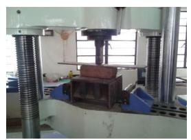
Figure 5. Testing of brick using 50T Universal Testing machine (UTM)
