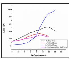
Figure 9. 5mm Sisal Fibre at 0.5, 1 and 1.5%
