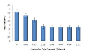
Figure 2. Effect of L-AA in different amounts on the free fluid content of cement slurry at  $52^{\circ}C$
