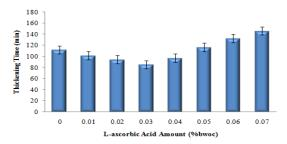
Figure 4. Thickening Time vs. amount of L-AA used in slurries at  $52^{\circ}C \& 5160 psi$
