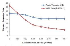
Figure 3. Effect of L-AA in different amounts on the rheology properties of cement slurry at  $52^{\circ}$  C
