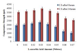
Figure 5. Compressive Strength for 8 and 24 hours vs. amount of L-AA used in slurries at  $60^{\circ}C$
