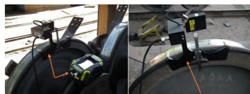
Figure 2. The laser view instrument (indicated by arrows) to measure the wheel profiles
