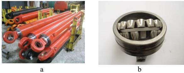
**Figure 1.** (a) Hydraulic cylinder of the truck crane and (b) bearing of the hinge-lever mould oscillator of the continuous casting machine
