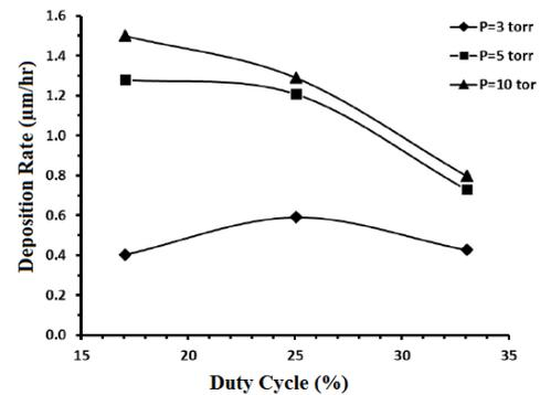
**Figure 2.** Effect of duty cycle on tantalum deposition rate under different total pressures
