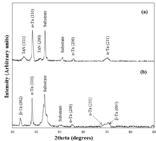
**Figure 4.** XRD patterns of Ta coating on TaN seed layer and (b) Ta single layer
