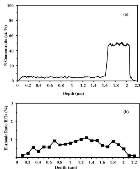
**Figure 5.** NRA results for PACVD Ta/TaN films as a function of (a) nitrogen and (b) hydrogen depth profile
