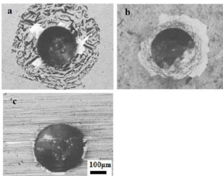
**Figure 7.** Qualitative adhesion test for film grown at (a) 5 torr pressure and 17% duty cycle with a  $\beta$ - rich monolayer Ta film, (b) the film that grown at 5 torr pressure and 25% duty cycle with a  $\alpha$ - rich monolayer tantalum film and (c) TaN/Ta bilayer indicating the maximum alpha content
