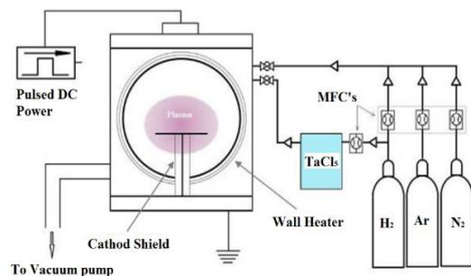
Figure 1. Schematic of Pulse DC-PACVD process
