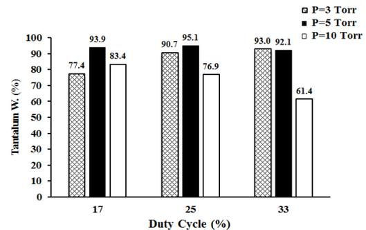
**Figure 3.** Purity of PACVD tantalum coatings deposited at various duty cycles and total pressures obtained from EDS elemental analysis
