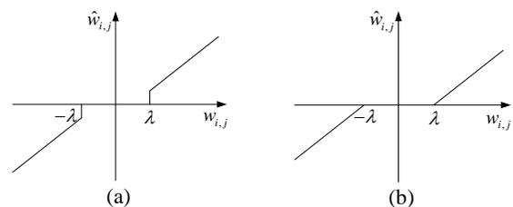
Figure 3. Threshold functions: (a) Hard threshold function and (b) Soft threshold function
