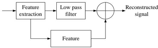
Figure 2. The schematic diagram of wavelet denoising
