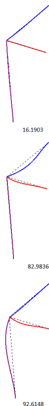
Figure 7. The first three natural frequencies and mode shapes of the coupled space frame with different properties
