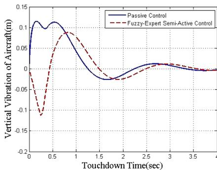
Figure 13. The vibration domain of aircraft under normal landing
