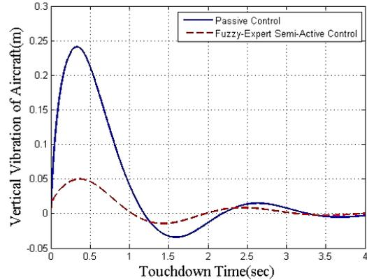
Figure 9. The vibration domain of aircraft under normal landing
