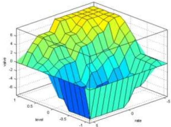
Figure 8. Surface view of rules (optimal trimf)
