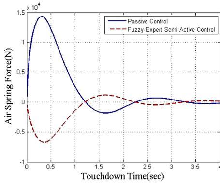
Figure 12. The impact force of aircraft under hard landing
