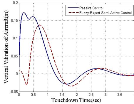
Figure 14. The vibration domain of aircraft under hard landing
