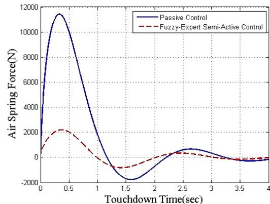
Figure 11. The impact force of aircraft under normal landing
