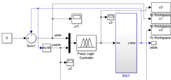
**Figure 4.** simulink model of Fuzzy controller for semi-active landing gear
