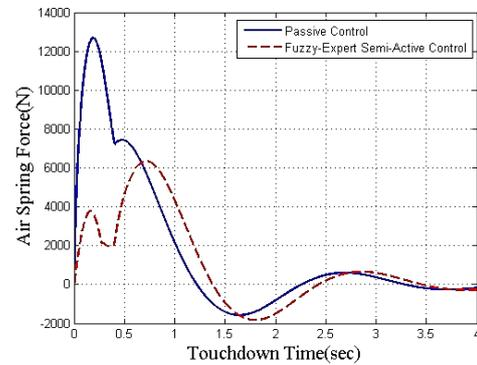
Figure 16. The impact force of aircraft under hard landing
