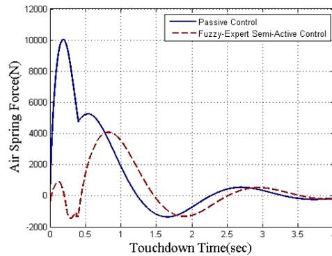
Figure 15. The impact force of aircraft under normal landing
