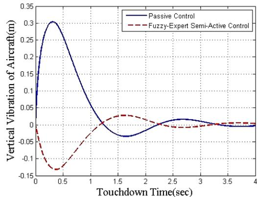
Figure 10. The vibration domain of aircraft under hard landing
