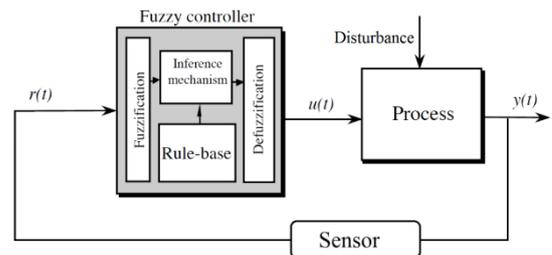
**Figure 1.** Block diagram of a fuzzy logic system
