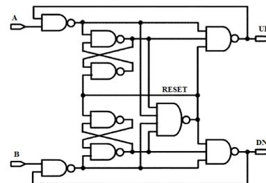
Figure 3. Gate level implementation of conventional PFDs [10]
