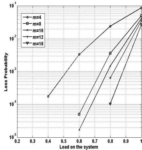
Figure 4. Packet loss probability vs. load (Random Traffic)
