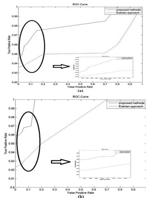
**Figure 10.** ROC curves obtained for (a) video so-called baby and (b) for video so-called shadow. Proposed method (solid line-blue), EVM (red dashed-line).
