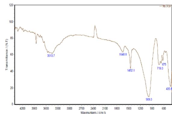
Figure 3. FTIR spectrum of sodalite zeolite
