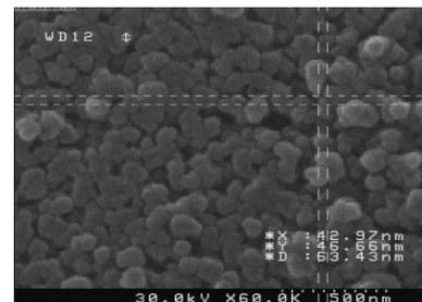
Figure 2. Scanning electron micrographs of sodalite zeolite
