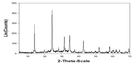
Figure 1. X-ray diffraction of synthesized sodalite zeolite.
