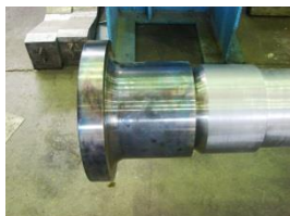
Figure 4. Installing a new shrink fit coupling on the rotor end
