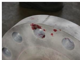
Figure 2. Penetration test result after refurbishing by welding and machining procedure
