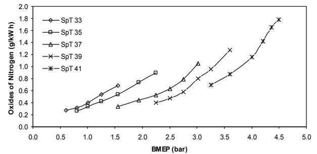
Figure 5. Variation of oxides of nitrogen emission at various spark timings
