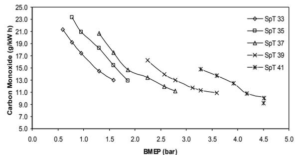
Figure 6. Variation of carbon monoxide emission at various spark timings
