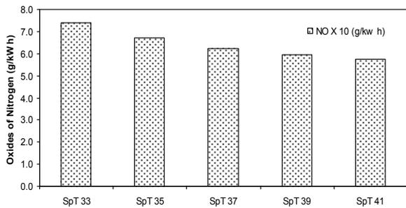
Figure 12. Variation of oxides of nitrogen at 3 bar BMEP for various spark timings
