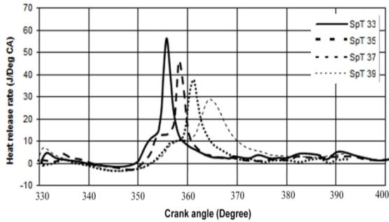
Figure 10. Variation of heat release rate patterns at 3 bar BMEP for various spark timings
