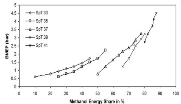
**Figure 3.** Energy share of hydrous methanol at various spark timings
