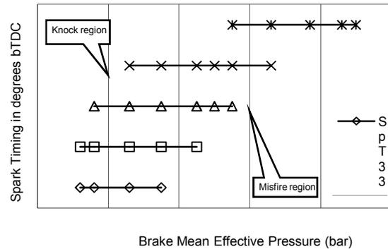
**Figure 2.** Operating range of hydrous methanol HCCI engine at various spark timings
