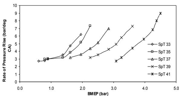
**Figure 8.** Variation of rate of pressure rise at various spark timings
