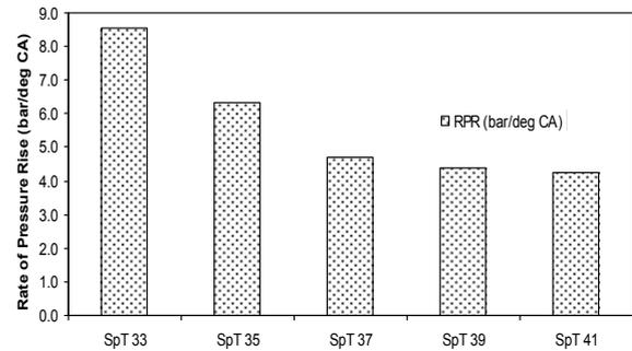
Figure 15. Variation of rate pressure rise at 3 bar BMEP for various spark timing
