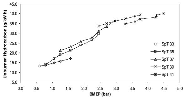
**Figure 7.** Variation of unburned hydrocarbon emission at various spark timings
