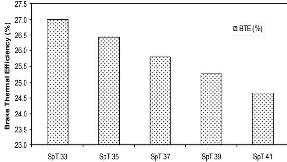
Figure 11. Variation of brake thermal efficiency at 3 bar BMEP for various spark timings
