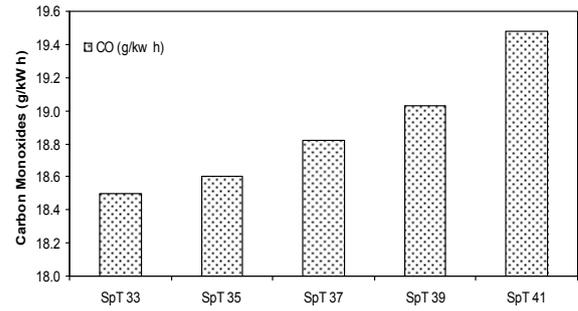
Figure 13. Variation of carbon monoxide at 3 bar BMEP for various spark timings
