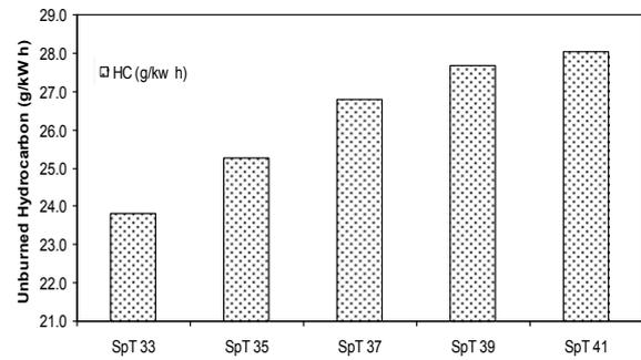
Figure 14. Variation of unburned hydrocarbon at 3 bar BMEP for various spark timings
