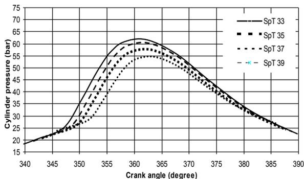
**Figure 9.** Variation of cylinder pressure at 3 bar BMEP for various spark timings
