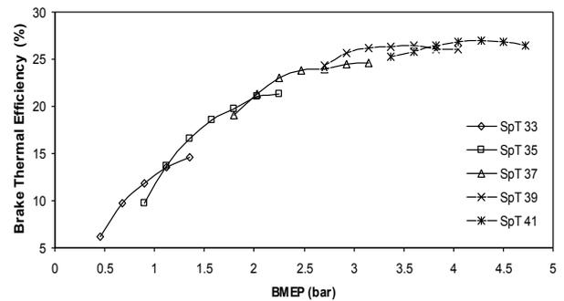
Figure 4. Variation of brake thermal efficiency at various spark timings
