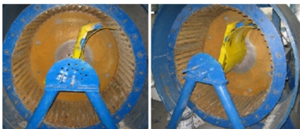
Figure 3. Measuring the cataract load mechanism
