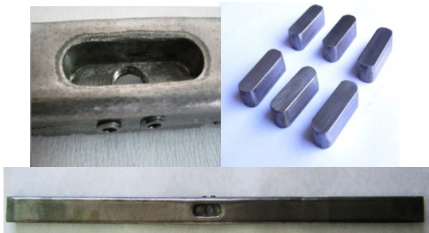
Figure 6. Specimens and their positions in liner face
