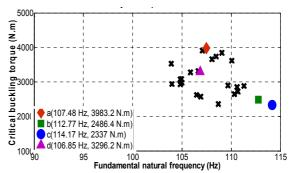
**Figure 8.** Critical buckling torque versus fundamental natural frequency in 3-objective optimization
