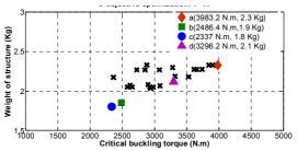
Figure 10. Total weight of structure versus critical buckling torque in 3-objective optimization
