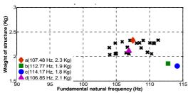
**Figure 9.** Total weight of structure versus fundamental natural frequency in 3-objective optimization
