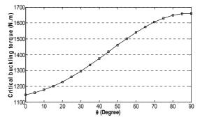
**Figure 5.** Effect of fiber orientation angle ( $\theta$ ) on critical buckling torque of stacking [ $\pm 45_{glass}/O_{carbon}/\theta_{glass}$ ]
