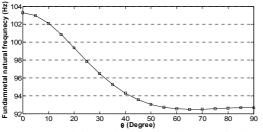
**Figure 2.** Effect of fiber orientation angle ( $\theta$ ) on fundamental natural frequency of stacking [ $\pm 45_{glass}/\theta_{carbon}/\theta_{glass}$ ]
