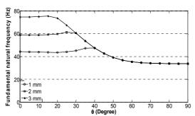
**Figure 3.** Effect of ply thickness on fundamental natural frequency.  $\theta$  is changing between 0 to 90 degree in  $[\pm \theta_{\text{glass}}]_2$  stacking. Legend shows the total thickness of composite tube
