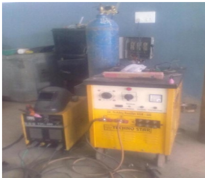
Figure 2. TIG welding set-up
