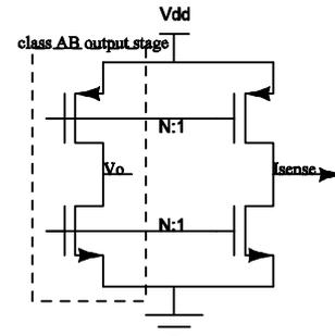
Figure 6. Current Sense Circuit
