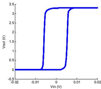
Figure 11. Voltage transfer curve of the designed hysteresis comparator
