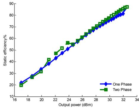
**Figure 18.** Simulated static efficiency of the envelope modulator versus DC output power
