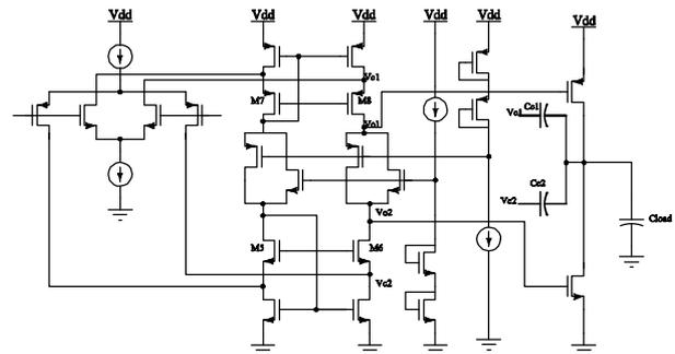
Figure 3. Class AB power amplifier architecture
