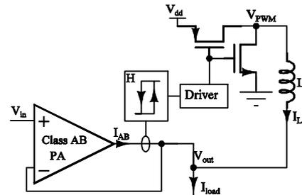
Figure 2. Block diagram of HSEM
