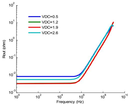
Figure 4. Simulated output impedance of class AB PA versus frequency for different DC output voltages
