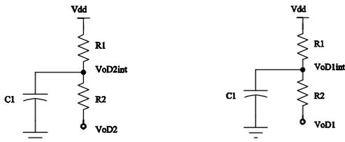
Figure 9. Integrator circuits used for integrating the switching voltages
