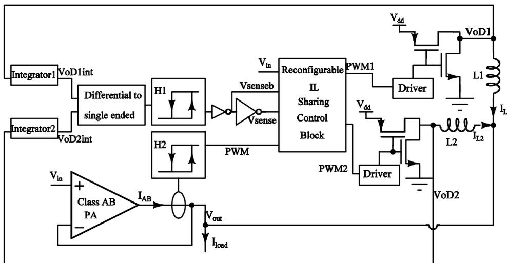
Figure 8. Block diagram of the proposed hysteretic two-phase envelope modulator.
