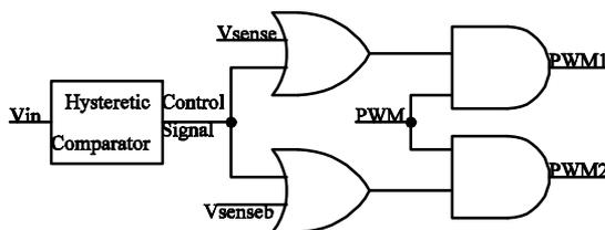
Figure 12. Reconfigurable IL sharing control block
