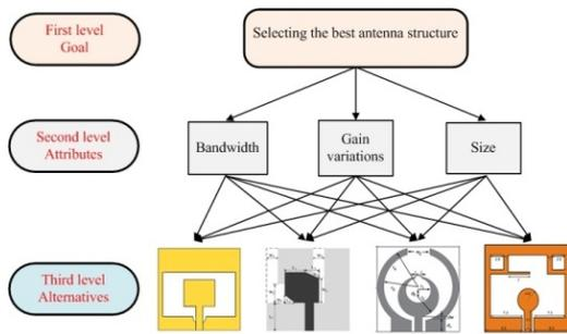
**Figure 9.** Analytical hierarchy schematic of the antenna selection problem.
