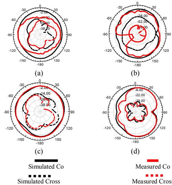
**Figure 8.** (a) H-plane (xz plane) pattern at 7 GHz, (b) E-plane (yz plane) pattern at 7 GHz, (c) H-plane (xz plane) pattern at 12 GHz and (d) E-plane (yz plane) pattern at 12 GHz.
