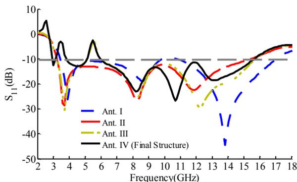
**Figure 3.**  $S_{11}$  curves for the step-by-step antennas
