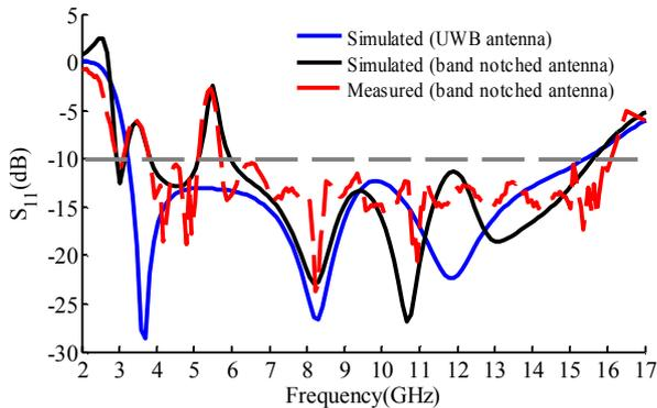
**Figure 5.** Simulated and measured  $S_{11}$  curves for the UWB and band notched antenna.
