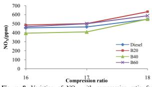
Figure 8. Variation of  $NO_X$  with compression ratio for different blends of biodiesel
