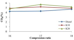
**Figure 3.** Variation of  $CO_2$  with compression ratio for different neat karanja oil blends
