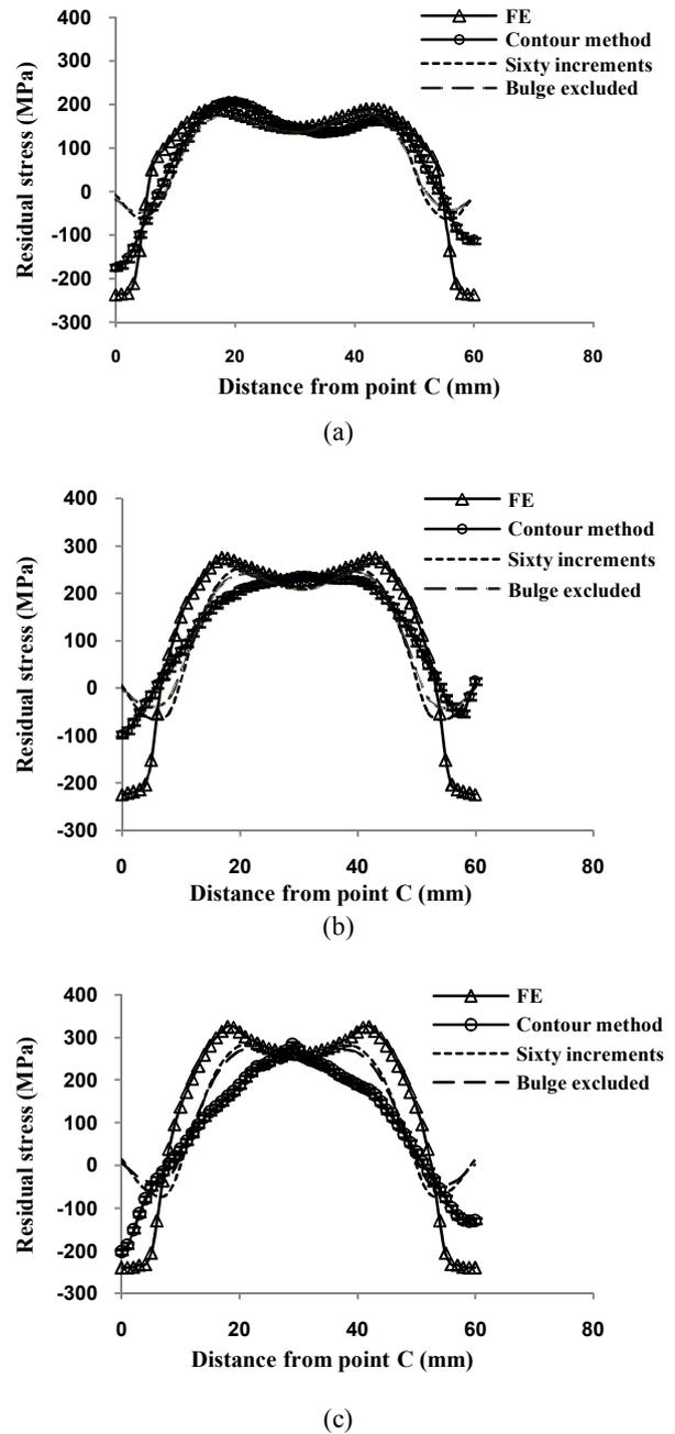
**Figure 13.** Residual stresses obtained by experimental approach, simulation of cutting in 60 increments and without bulge error in comparison with those predicted by finite element along axis of cylinder (line CD) at (a) 500°C, (b) 700°C and (c) 850°C
