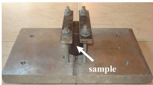
Figure 3. Fixture and clamping of the sample
