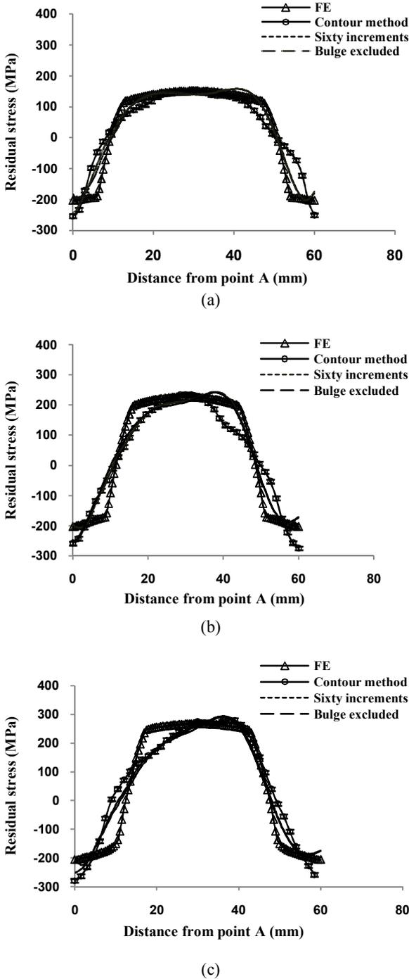
**Figure 12.** Comparing all residual stress distributions along centerline of the cylinder (line AB) for the sample quenched at (a) 500°C, (b) 700°C and (c) 850°C
