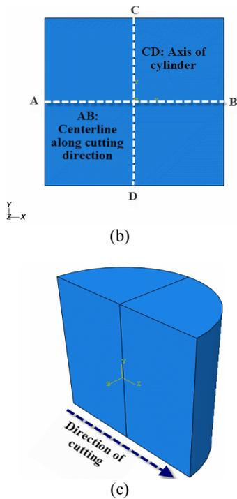
**Figure 6.** (a) The 3D finite element model of the half cylinder with exaggerated applied displacements by a factor of 70, (b) A schematic of centerline (line AB) and axis of model (line CD) and (c) cutting direction.
