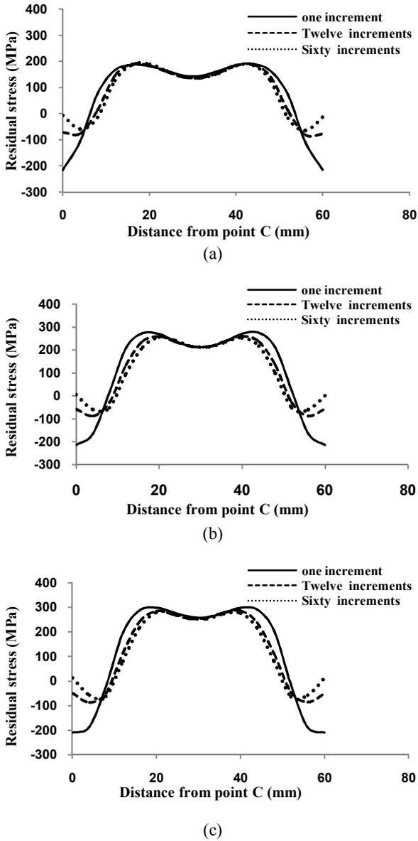
**Figure 10.** Obtained residual stresses by cutting in one, twelve and sixty increments along axis of cylinder (line CD) quenched at (a) 500°C, (b) 700°C and (c) 850°C
