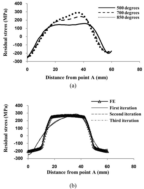
**Figure 11.** (a) Obtained residual stresses by simulation of cutting in 60 increments without bulge error along centerline of cylinder (line AB) at 500°C, 700°C and 850°C, (b) Residual stresses obtained by cutting simulation in first, second and third iterations of bulge errors excluding at 850°C along cylinder centerline (line AB) compared with FE prediction.
