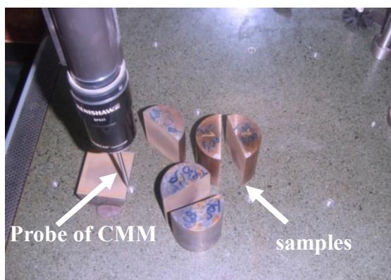
Figure 4. Measuring the deviation of cut surfaces by CMM
