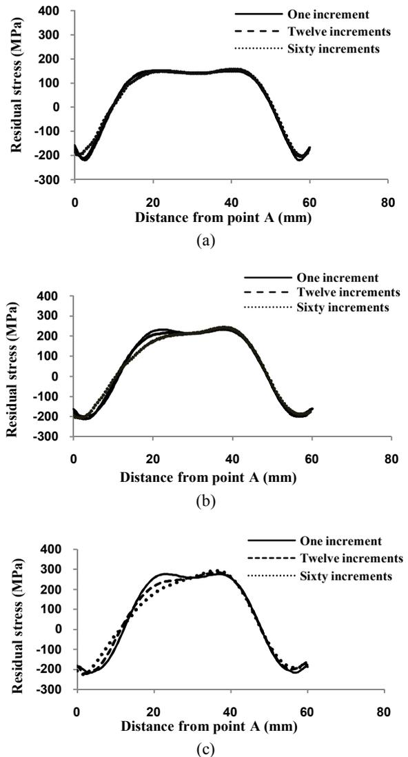
**Figure 9.** Obtained residual stresses by cutting in one, twelve and sixty increments along centerline of cylinder (line AB) quenched at (a) 500°C, (b) 700°C and (c) 850°C
