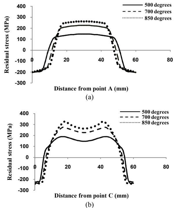
**Figure 8.** Residual stresses obtained from FE, (a) along centerline of cylinder (line AB) in three samples and (b) along axis of cylinder (line CD) in three samples
