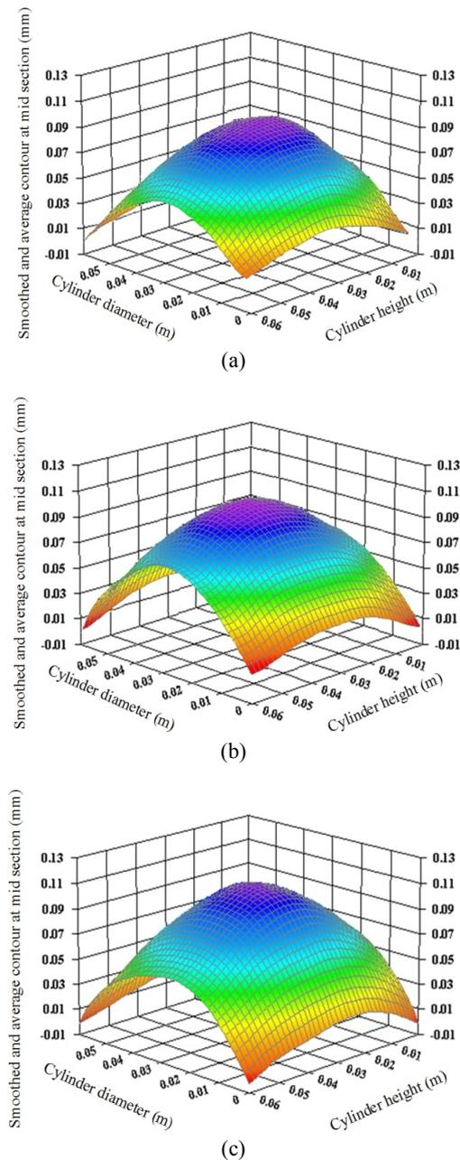
**Figure 5.** Averaged of smoothed contour in cut surface of cylinders quenched at (a) 500°C, (b) 700°C, (c) 850°C.
