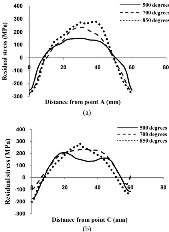
**Figure 7.** Residual stresses obtained by contour method in three samples, (a) along line AB and (b) along axis of cylinder (line CD).
