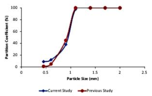
**Figure 13.** Comparison of simulated partition curve plotted for overflow stream with that of obtained in previous studies for the first plate with a slope of 28 degree
