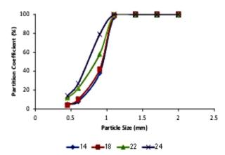
Figure 9. Partition curve of screen overflow with change in the slope of the second plate
