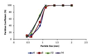
Figure 10. Simulated partition curves for particles recovered to overflow stream for third screening plate at various slopes
