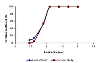
**Figure 11.** Comparison of simulated partition curve plotted for particles recovered to overflow stream with that of previous studies with vibration amplitude equal to 1.5 mm
