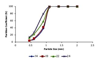
Figure 9. Partition curve of screen overflow with change in the slope of the second plate
