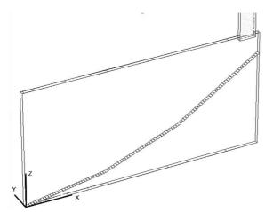
**Figure 2.** Generated virtual screen in PFC3D software. The feeding part of the screen containing the various balls as the feed particles can be seen at the top right of the figure.
