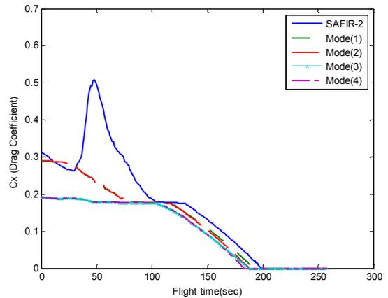
Figure 8. Launch vehicle drag coefficient ( $C_x$ ) vs. time
