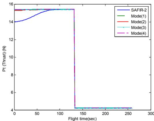
Figure 7. Launch vehicle thrust vector vs. flight time
