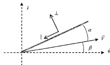
Figure 2. Representation offers acting on plate while at angle alpha
