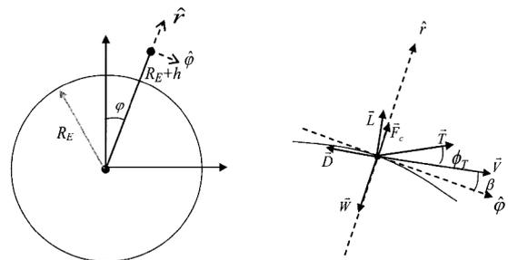
Figure 1. Representation of forces acting on vehicle
