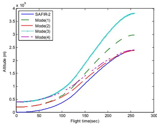
Figure 5. Launch vehicle altitude vs. flight time
