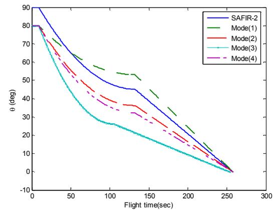
Figure 9. Launch vehicle Pitch angle ( $\theta$ ) vs. flight time
