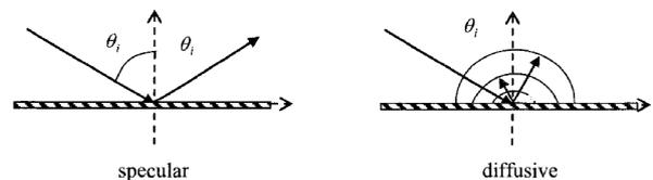
Figure 4. Specular and diffuse reflection
