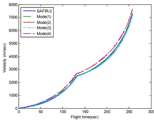
Figure 6. Launch vehicle velocity vs. flight time
