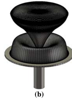
Figure 21. (a) The third optimized profile for UWB monopole antenna with finite ground plane (the volcano smoke antenna) and (b) the 3-D view of antenna
