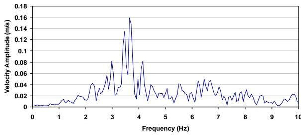
**Figure 6.** Velocity response of a point at the top of silo in frequency domain in model 2
