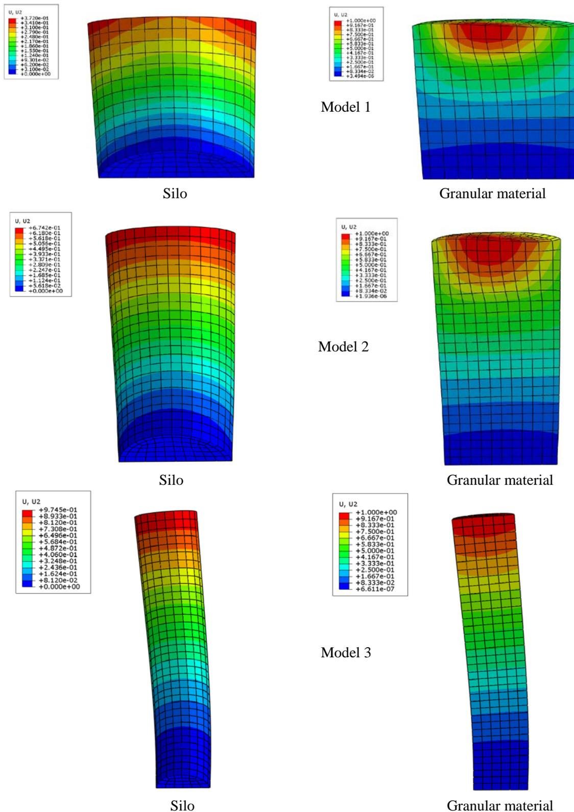
**Figure 8.** The deformed shapes of silo and granular material inside silo in the first translational mode computed by eigenvalue analysis considering four layers of granular material with elastic behavior
