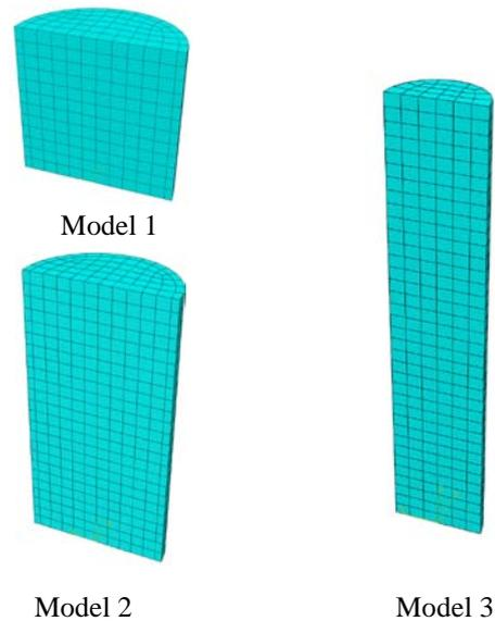
**Figure 2.** The Finite element mesh of silo models and granular material
