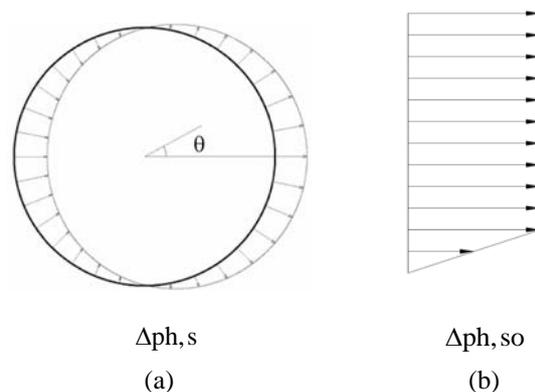
**Figure 1.** (a) The distribution of  $\Delta p_{h,s}$  in the section of silo, (b) The distribution of  $\Delta p_{h,so}$  in the height of silo
