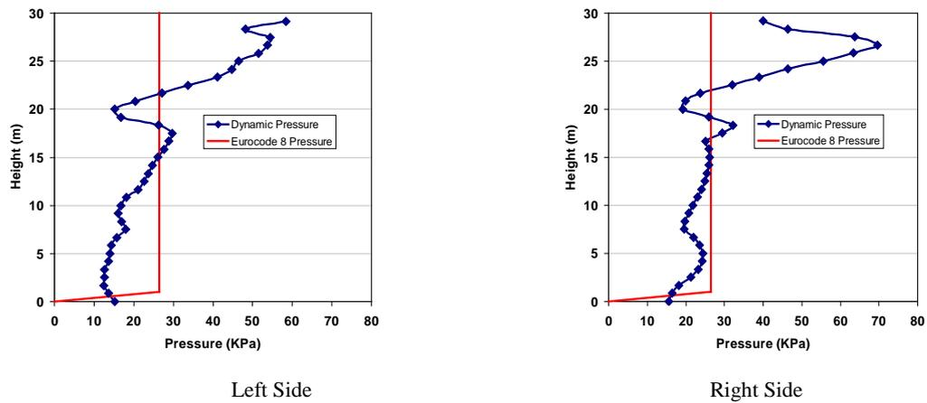
**Figure 11.** The distribution of dynamic pressure envelopes versus height in direction of earthquake excitation for right and left sides of silo in model 3
