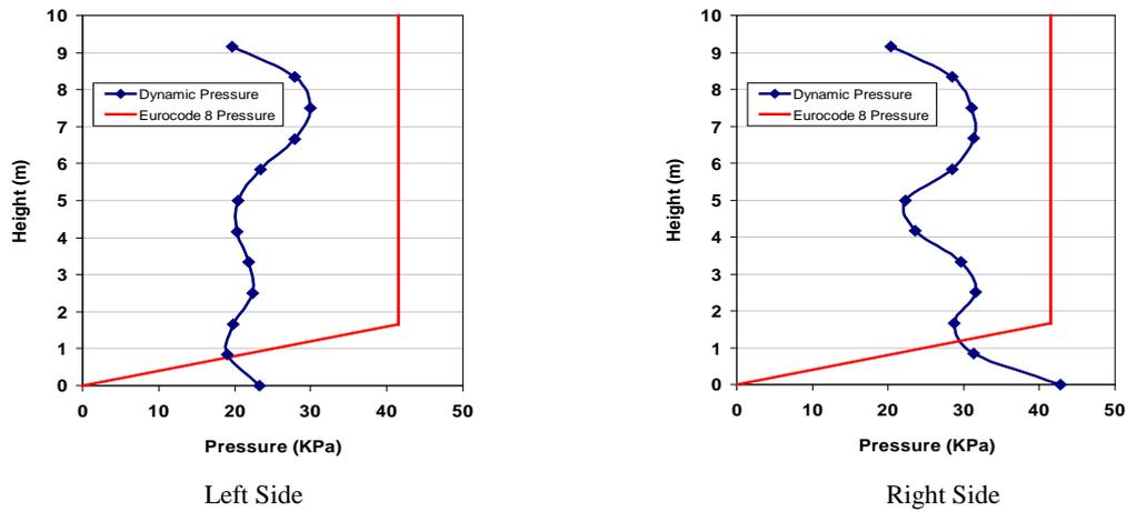
**Figure 9.** The distribution of dynamic pressure envelopes versus height in direction of earthquake excitation for right and left sides of silo in model 1
