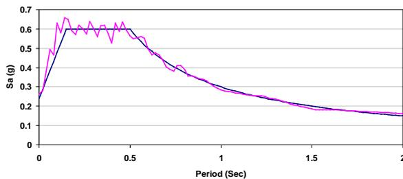
**Figure 4.** Response spectrum of earthquake excitation generated by SeismoMatch
