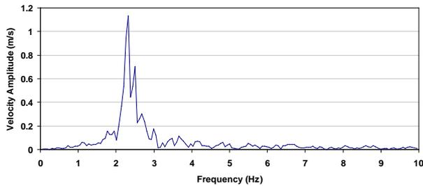
**Figure 7.** Velocity response of a point at the top of silo in frequency domain in model 3
