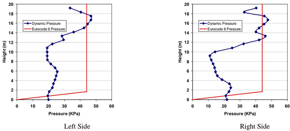
**Figure 10.** The distribution of dynamic pressure envelopes versus height in direction of earthquake excitation for right and left sides of silo in model 2
