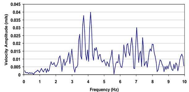
**Figure 5.** Velocity response of a point at the top of silo in frequency domain in model 1
