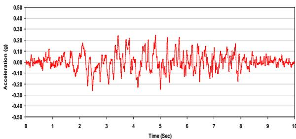
**Figure 3.** Earthquake acceleration applied to the silo models
