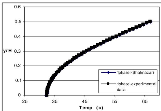
**Figure 8.** Comparison of temperature distributions considering Shahnazari's experimental correlation and Fried & Combarnous's experimental data for thermal dispersion.  $Pe = 10$  ,  $\xi = 0.3$
