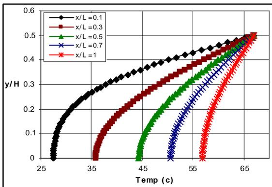
**Figure 3.** Comparison of temperature distribution in various dimensionless length of channel at constant Peclet number.  $Pe = 5$
