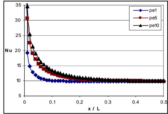
**Figure (12).** Peclet number effects on local Nusselt number which shows Nusselt number versus dimensionless length of channel at different Peclet number.
