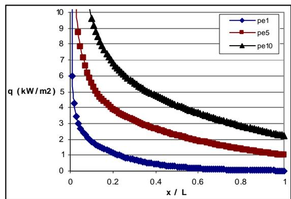
**Figure 14.** Peclet number effects on heat flux which shows heat transfer rate versus dimensionless length of channel at different Peclet number.
