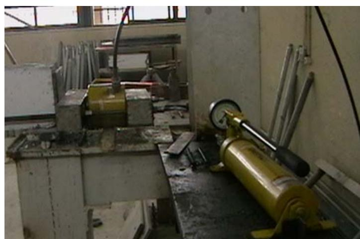
**Figure 4.** Post-tensioning using hydraulic jack
