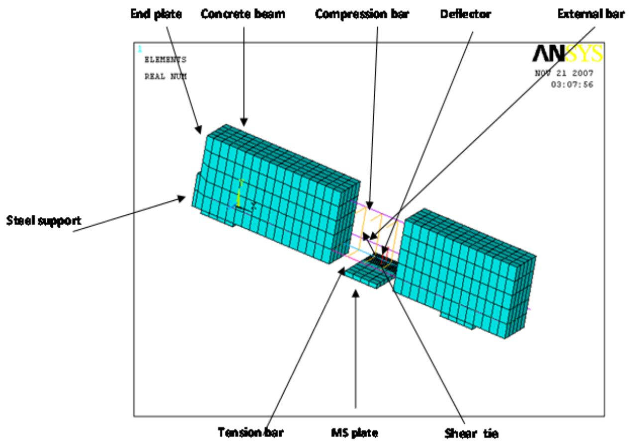
Figure 10. ANSYS beam model
