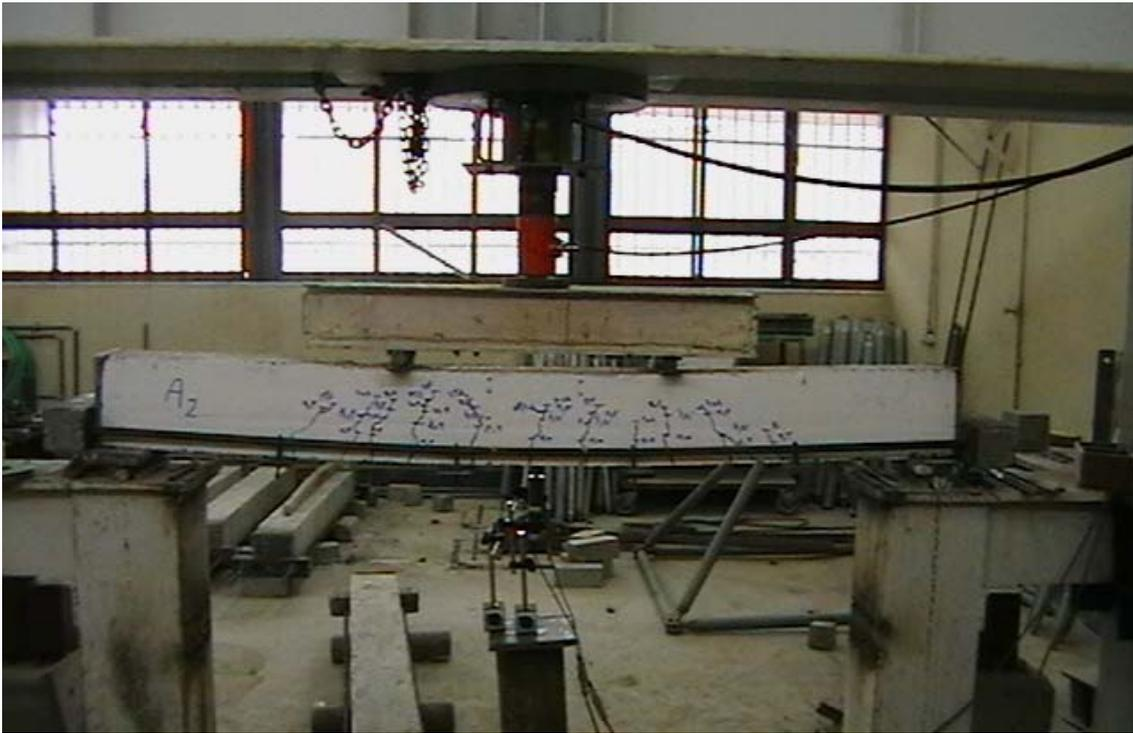
Figure5. Loading the beam
