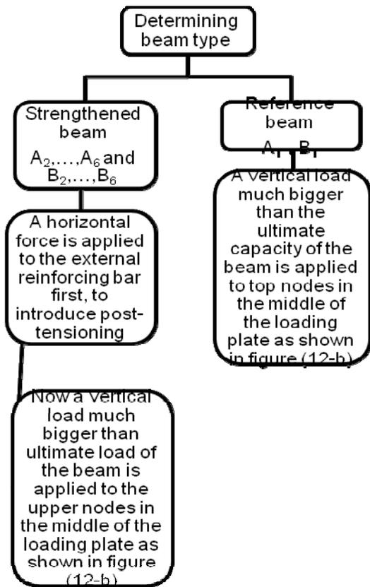
Figure 13. Algorithm of how applying loads
