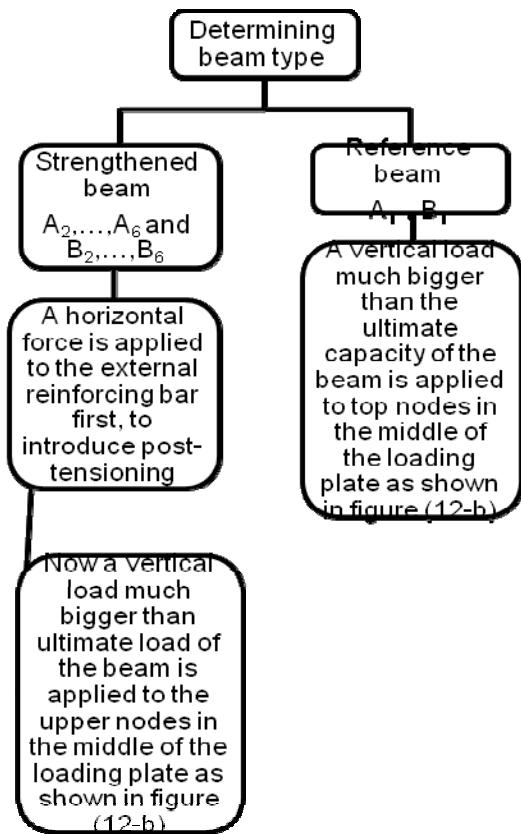
**Figure 13.** Algorithm of how applying loads
