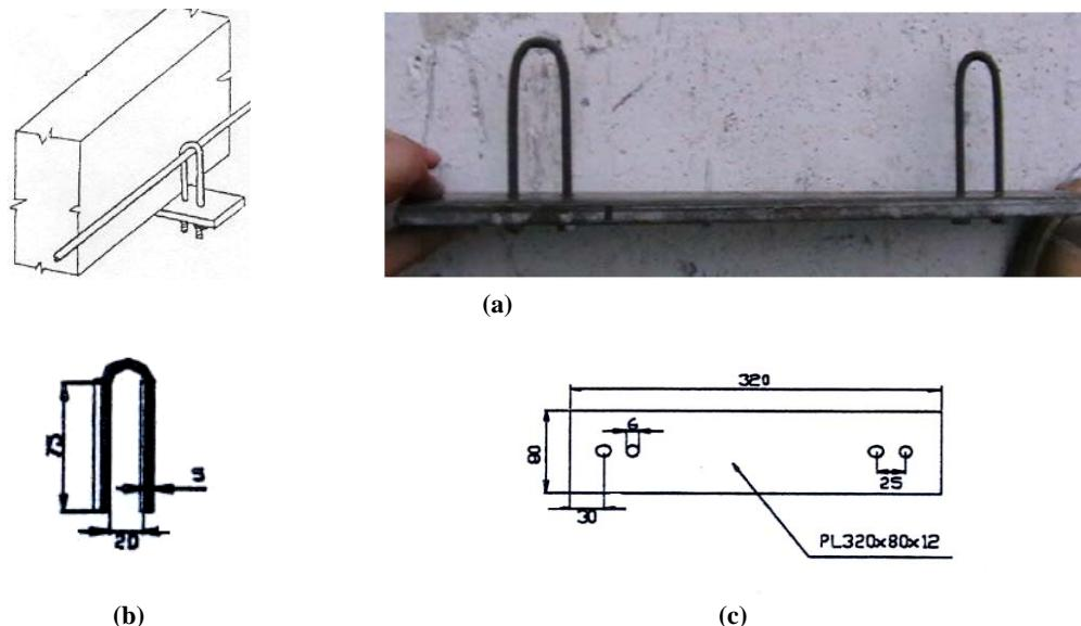
**Figure 3.** Details of deflectors; (a) Used in the lab; (b) Deflector; (c) MS strip
