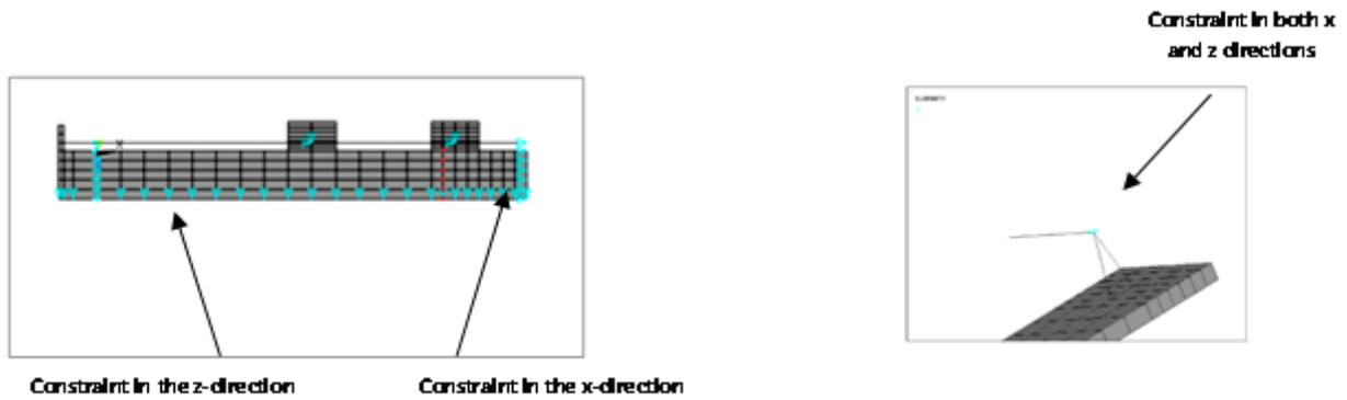
**Figure 11.** Boundary conditions for planes of symmetry and the point of attachment of external strengthening reinforcing bars and deflector
