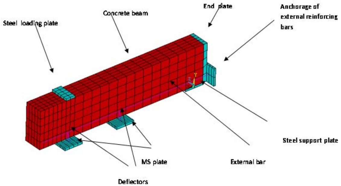
Figure9. Constituent elements of strengthened reinforced concrete beam in ANSYS
