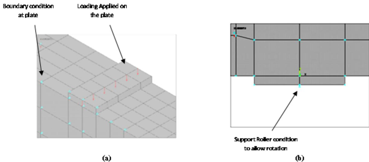
**Figure 12.** (a) boundary conditions of the support; (b) loading on the steel plates under concentrated load
