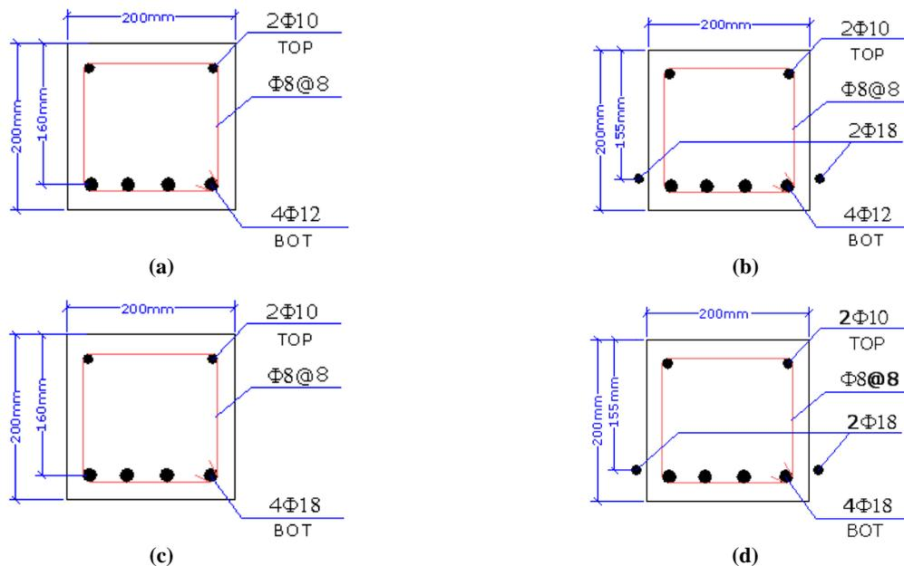
Figure 1. Cross sections of test beams, (a) beam A1; (b) beams A2 to A6; (c) beams B1; (d) beams B2 to B6
