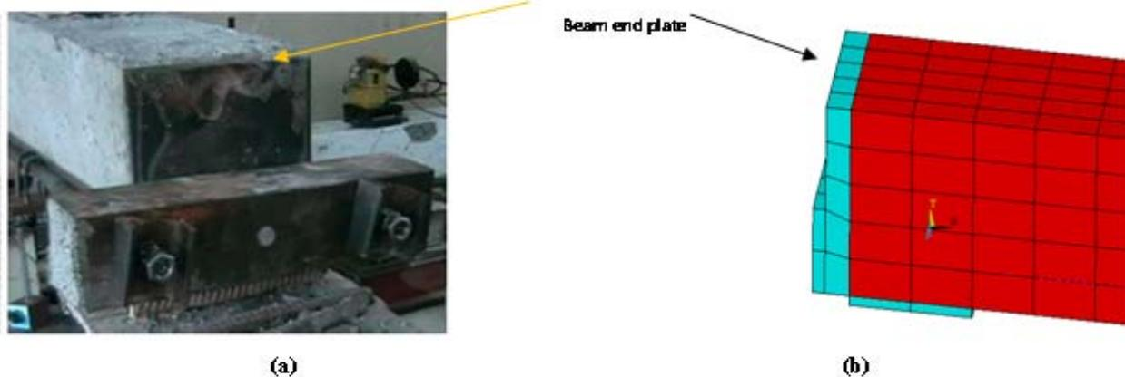
**Figure 7.** Beam end plates; (a) in test beams; (b) in the model
