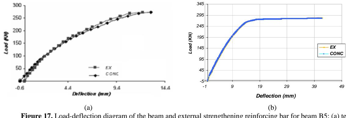
**Figure 17.** Load-deflection diagram of the beam and external strengthening reinforcing bar for beam B5; (a) test beam; (b) modeled beam
