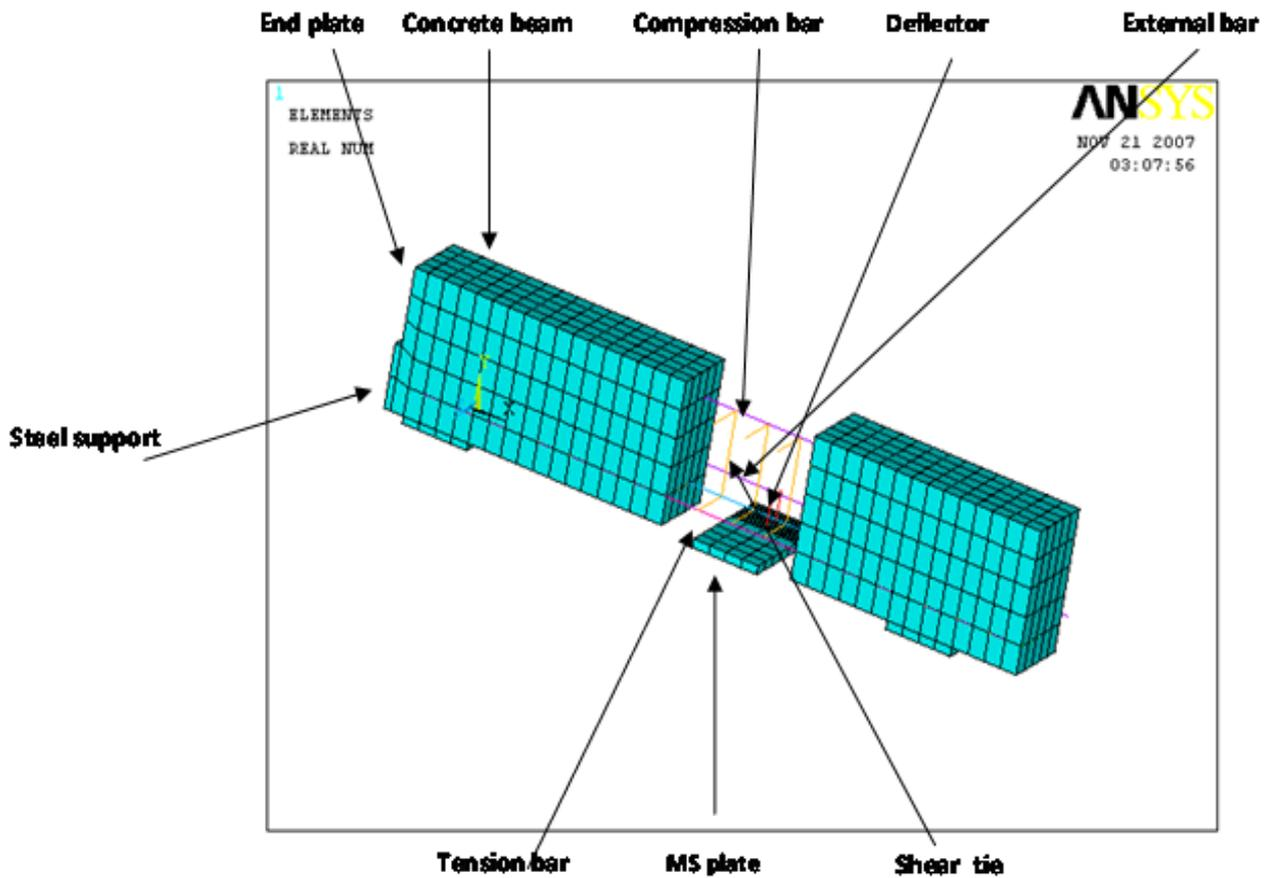
Figure 10. ANSYS beam model
