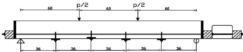
**Figure 2.** The position of deflectors of external reinforcing bars and the position of applied loads
