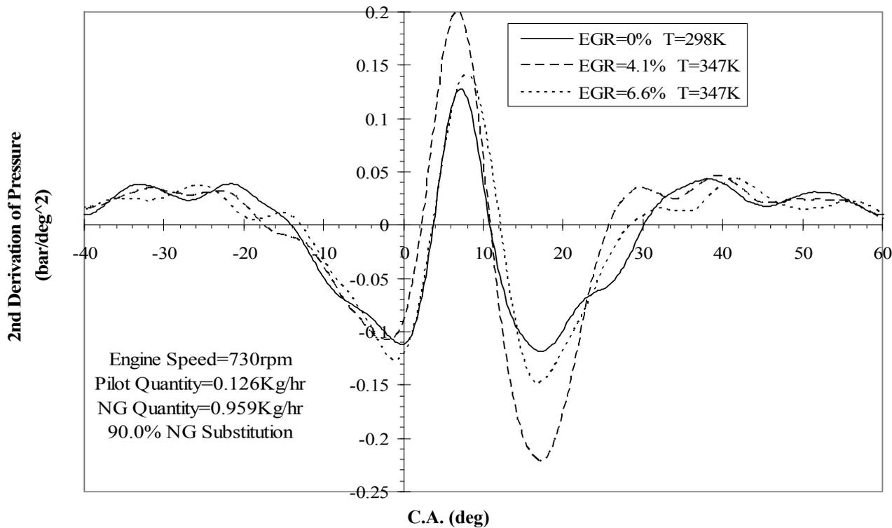
**Figure 6.** Variations of the 2<sup>nd</sup> derivative of cylinder pressure with crank position for constant intake mixture temperatures and different percentages of EGR at 10 and 50 percents of full load.
