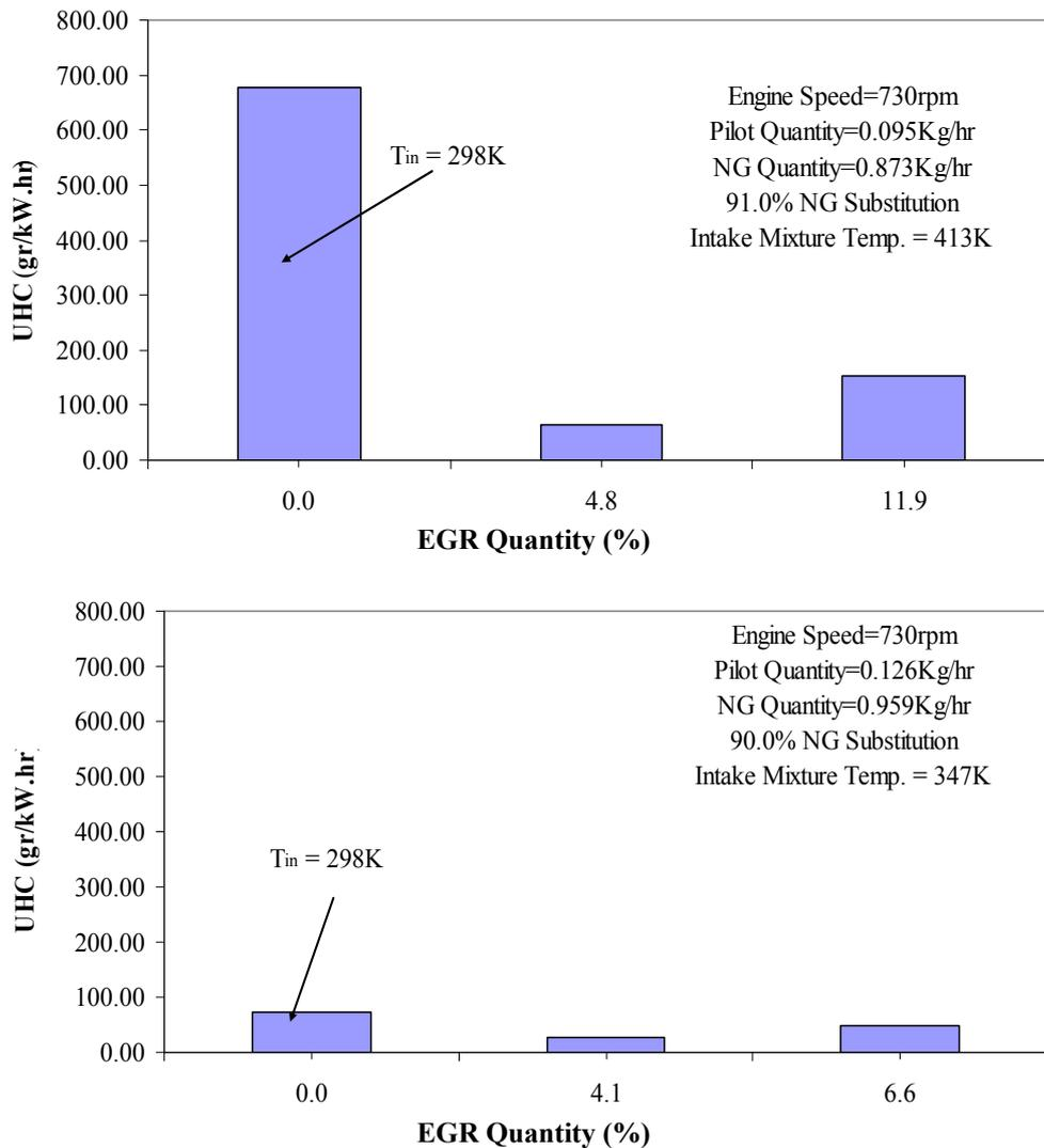
**Figure 9.** Variations of the unburned hydrocarbons emission with EGR percentage for constant intake mixture temperatures at 10 and 50 percents of full load.
