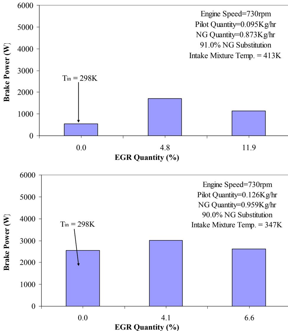
**Figure 7.** Variations of the brake power with EGR percentage for constant intake mixture temperatures at 10 and 50 percents of full load.
