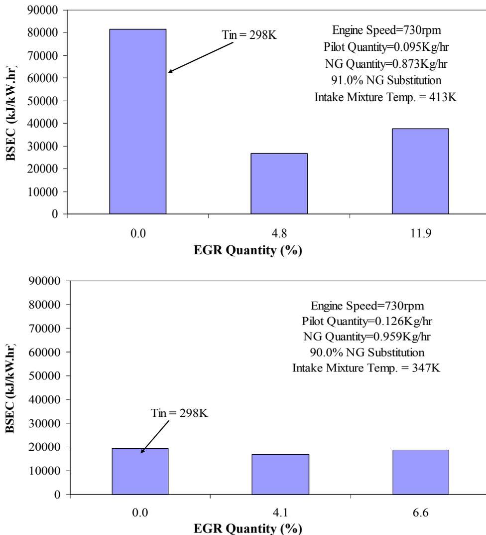
**Figure 8.** Variations of the brake specific energy consumption with EGR percentage for constant intake mixture temperatures at 10 and 50 percents of full load.
