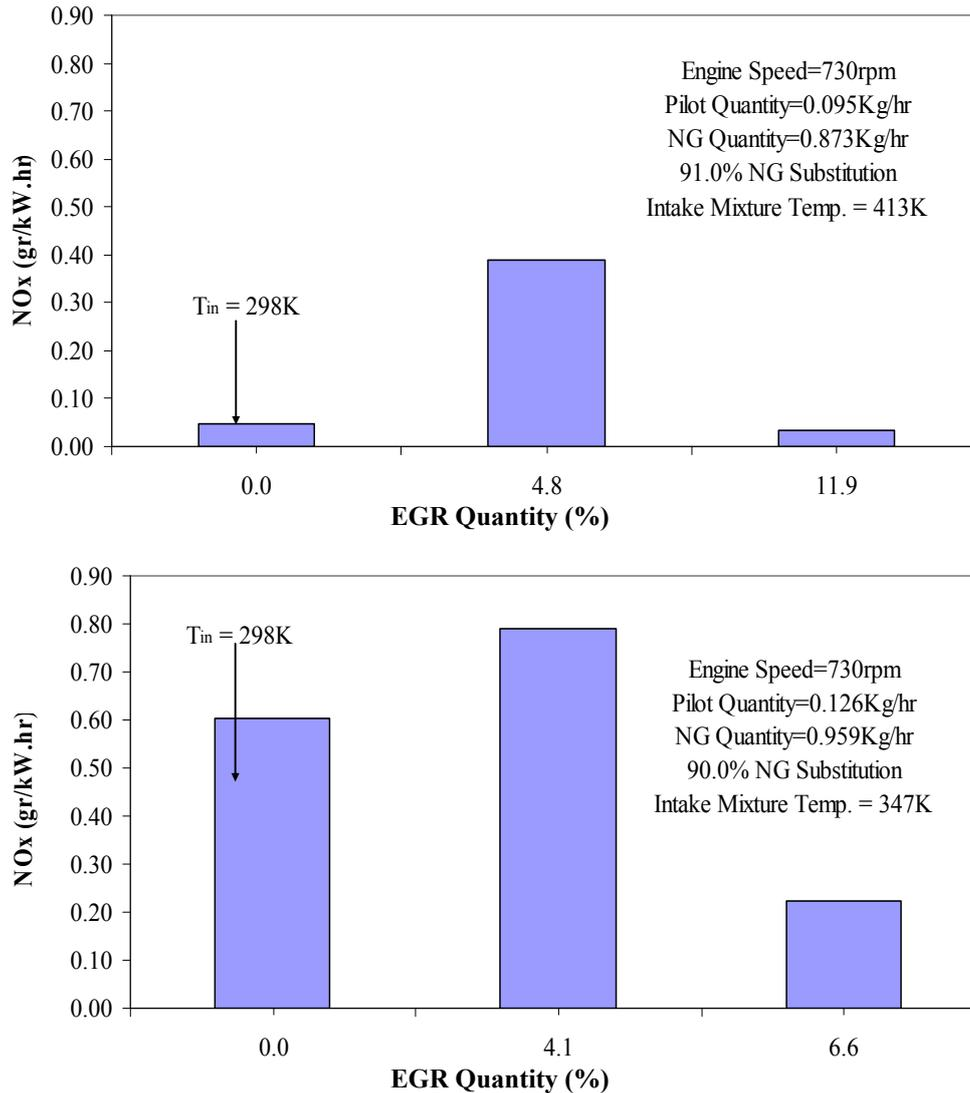
**Figure 11.** Variations of the nitrogen oxides emission with EGR percentage for constant intake mixture temperatures at 10 and 50 percents of full load.
