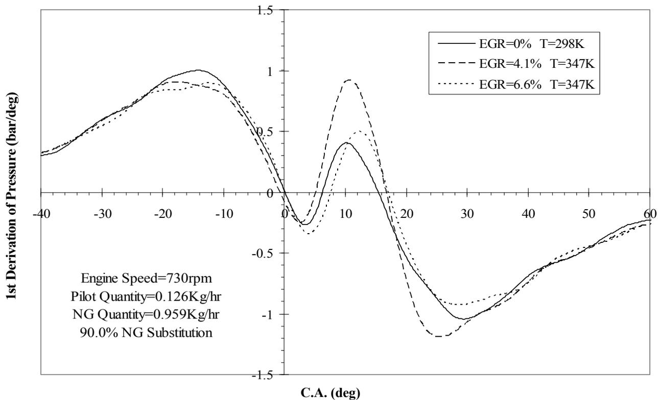
**Figure 5.** Variations of the 1<sup>st</sup> derivative of cylinder pressure with crank position for constant intake mixture temperatures and different percentages of EGR at 10 and 50 percents of full load.
