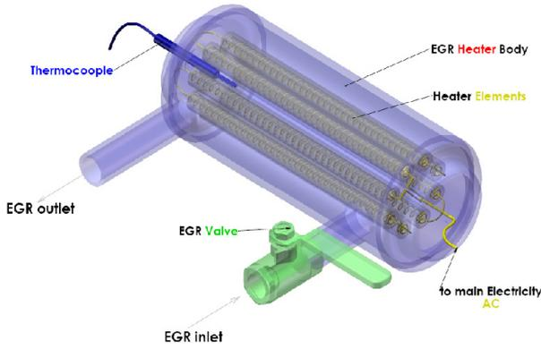
Figure 2. EGR electric heater layout.
