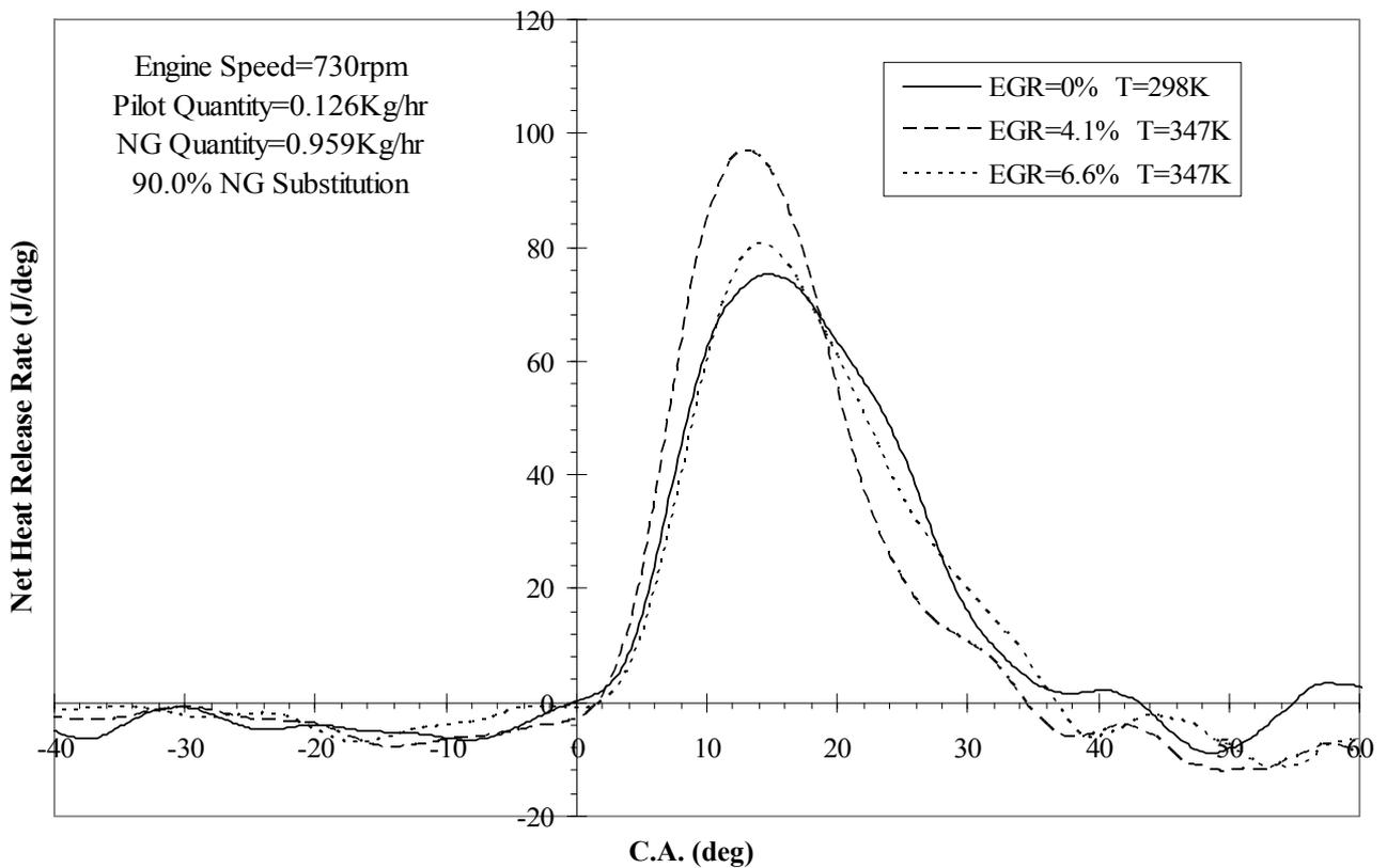
**Figure 4.** Variations of the net heat release rate with crank position for constant intake mixture temperatures and different percentages of EGR at 10 and 50 percents of full load.
