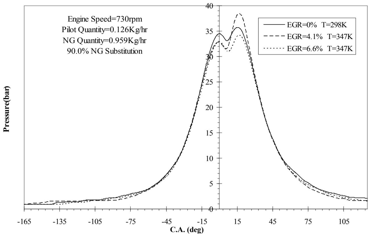
**Figure 3.** Variations of the cylinder pressure with crank position for constant intake mixture temperatures and different percentages of EGR at 10 and 50 percents of full load.
