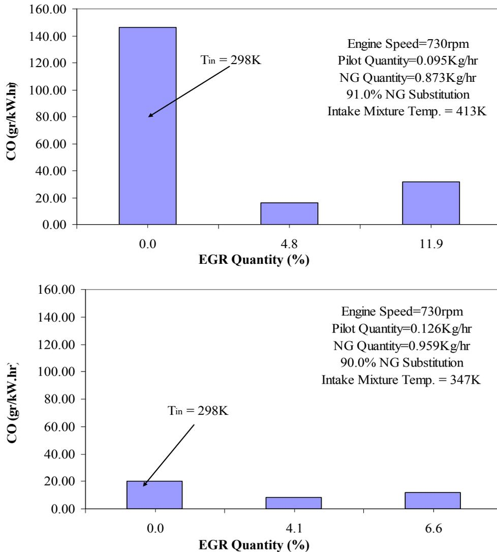
**Figure 10.** Variations of the carbon monoxide emission with EGR percentage for constant intake mixture temperatures at 10 and 50 percents of full load.
