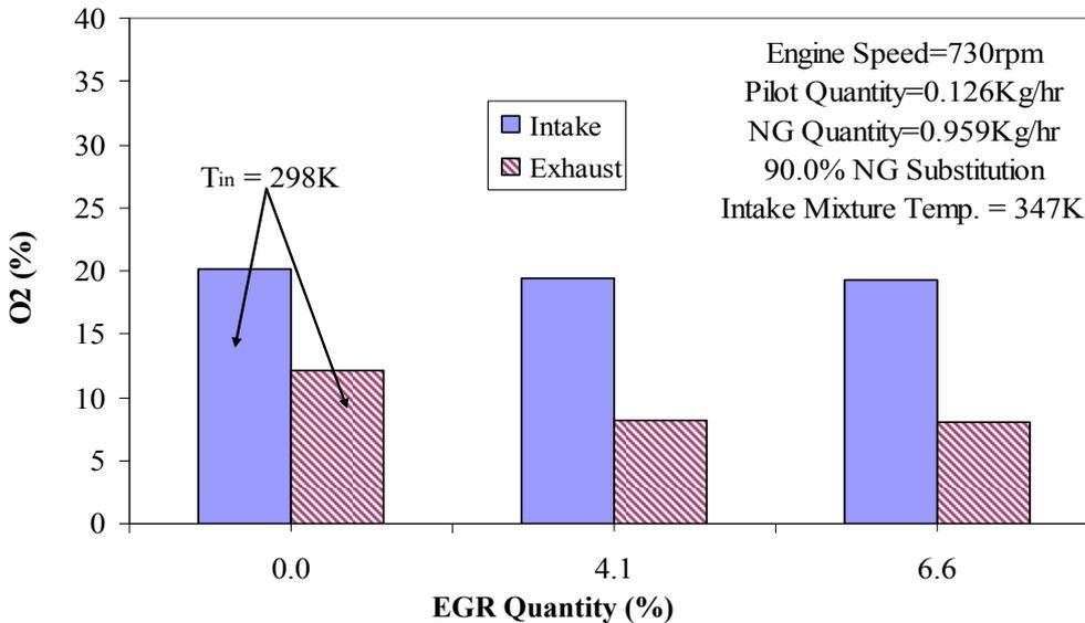
**Figure 12.** Variations of the intake and exhaust oxygen concentrations with EGR percentage for constant intake mixture temperatures at 10 and 50 percents of full load.
