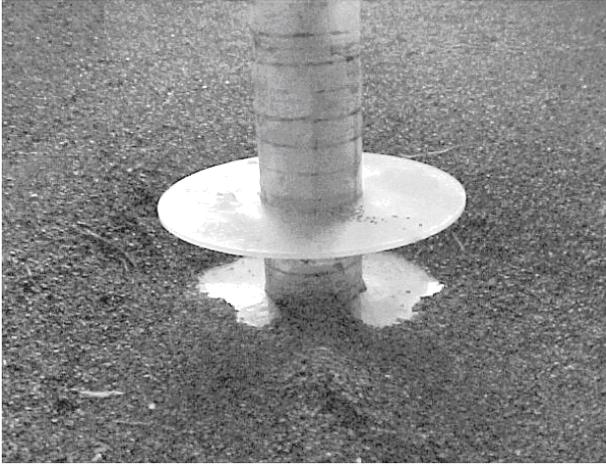
**Figure 6.** Scour hole around pier protected by two collar (Test No. 4)-looking downstream.
