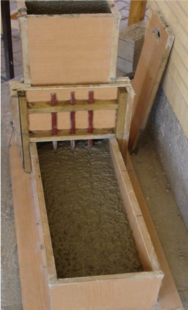
**Figure 3.** L-box test.
