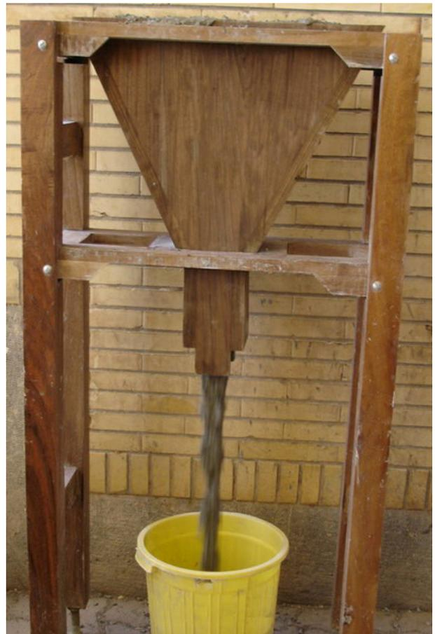
**Figure 4.** V-Funnel test.
