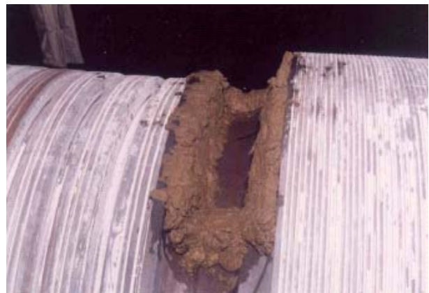
Figure 7. Utilization of locally hot spotting on bent rotor with moisture insulation.
