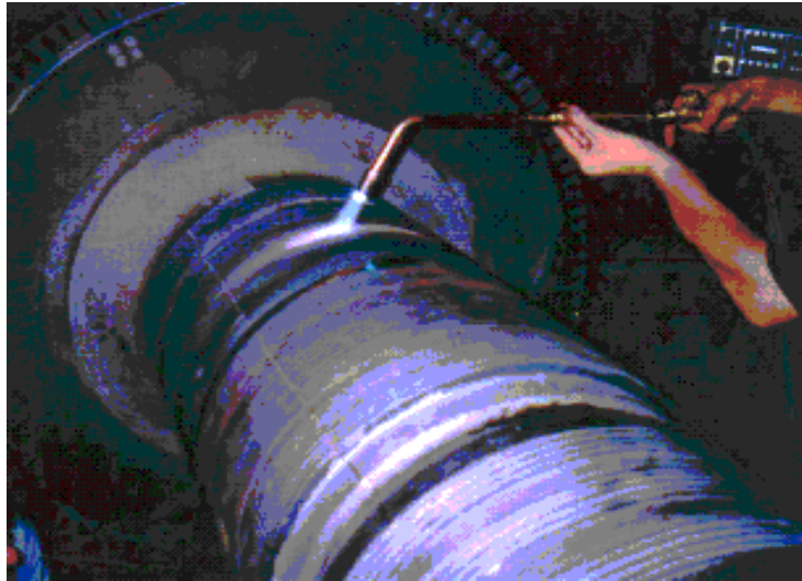
Figure 3. The mechanism of hot spotting heat treatment.
