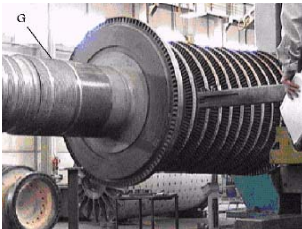
Figure 1. The bent rotor in shaft area (denoted by G).
