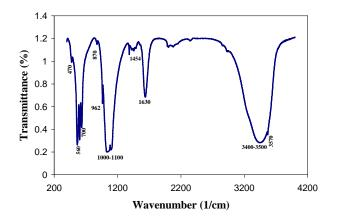
Figure 2. The FTIR spectrum of the HAp nanorods.
