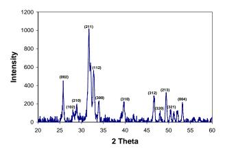
Figure 1. XRD pattern of the as-synthesized HAp nanorods.
