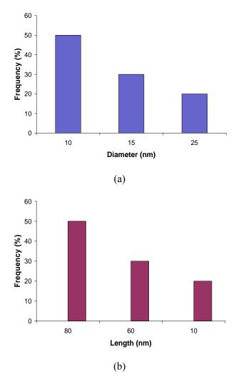
**Figure 5**. (a) Histogram of the nanorod diameter distribution and (b) histogram of the nanorod length distribution.
